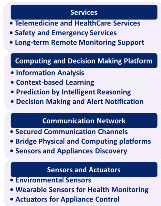
Figure 1.3 A four–layer architecture of the smart health–monitoring system [1.22].
