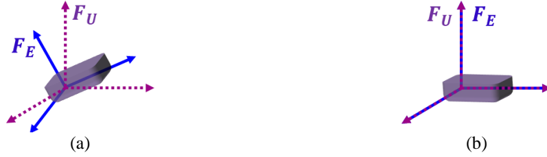
Figure 3.2 Aligning sensor frame to the earth frame assuming no rotation around the vertical z -axis.
