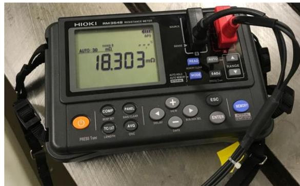
Fig. 4.10. Measurement of the phase winding resistance.
