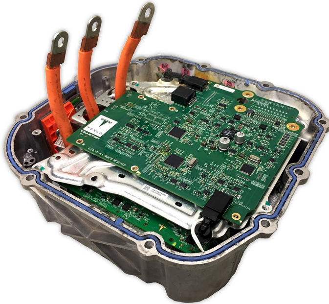
Figure 2.5: Tesla Model S dual motor rear drive unit inverter.
