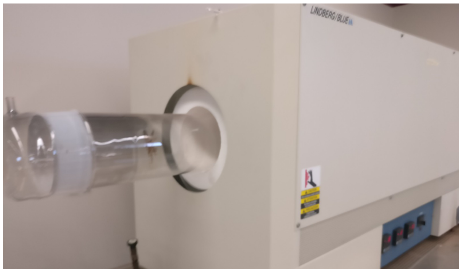
FIGURE 4.8: Photograph of Lindberg/Blue M TM tube furnace used in the annealing of 3 inch GeO 2 samples.
