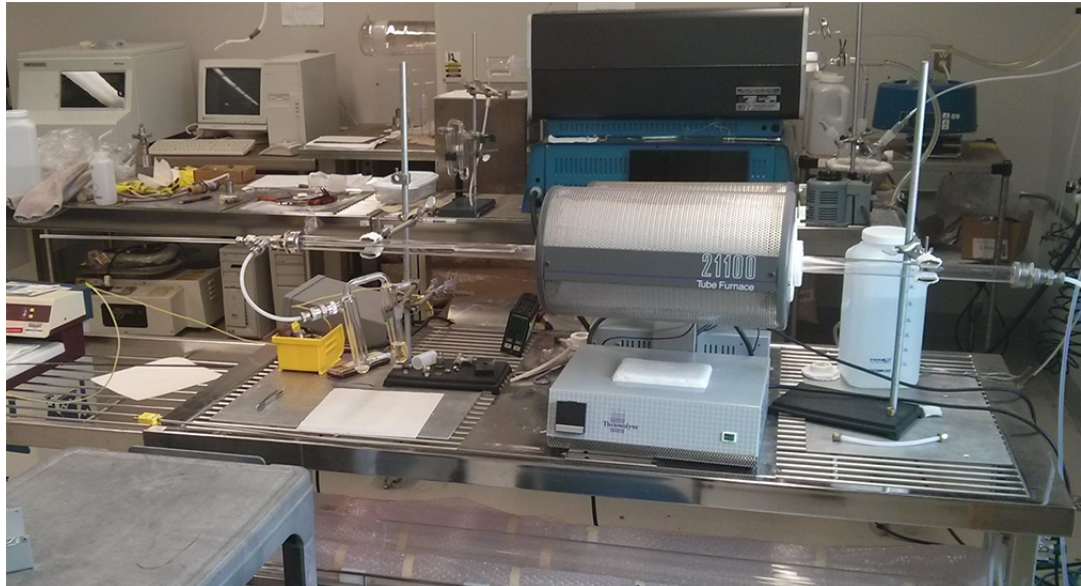
FIGURE 4.7: Photograph of Thermolyne™ F21100 tube furnace used in the annealing of rare-earth doped SiO x samples.
