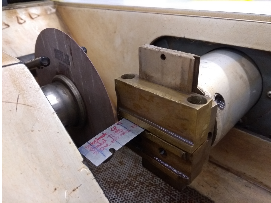
Figure 4.9: The sample prior to being cut in the precision cutter. Two jets of water are on either side of the blade.
