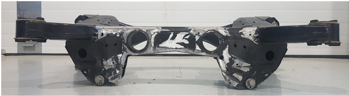
Figure 6.7: Rear cradle with modification cuts.
