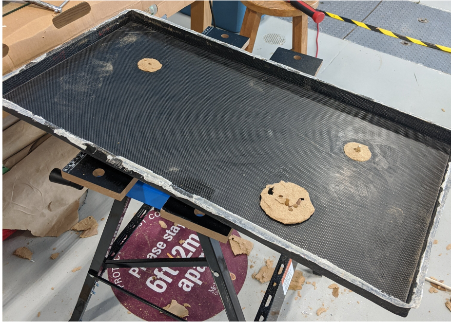
Figure 6.8: Battery enclosure carbon fiber lid, post infusion.
