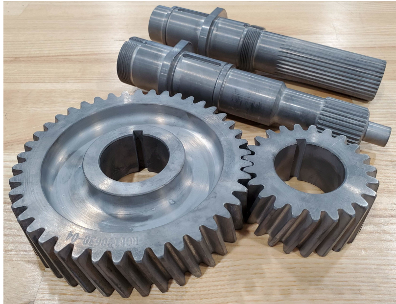
Figure 5.1: Wheel gear (left), pinion gear (right), and shafts as received from Rapid Precision Machining & Gearing Ltd
