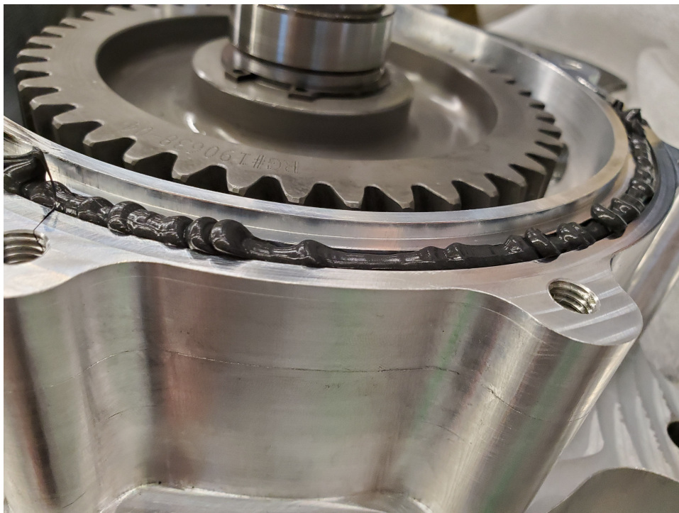
Figure C.5: Silicone placement in sealant groove.
