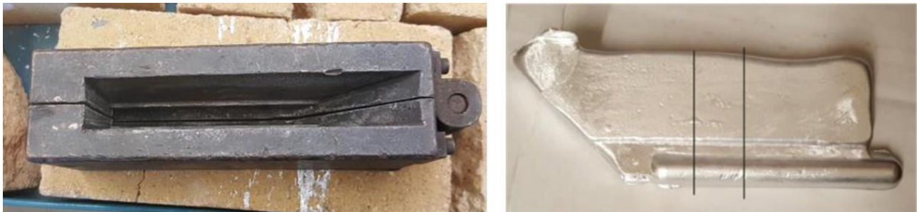
Figure 4.8: Copper mould and typical cast sample for alloy chemistry analyses using GDOES.
