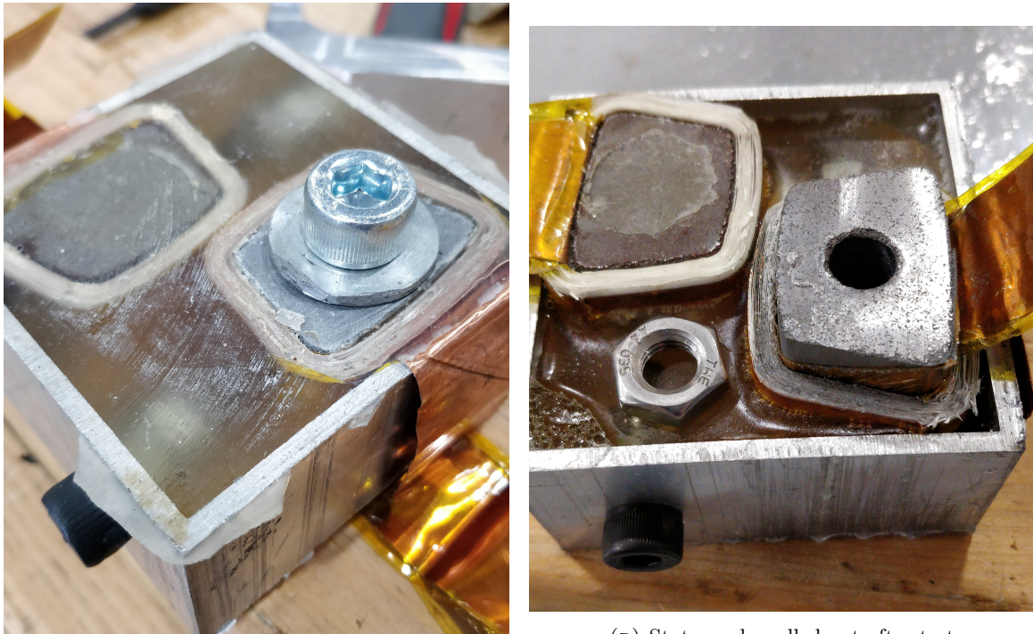
(A) Two stator poles encapsulated in test mold
