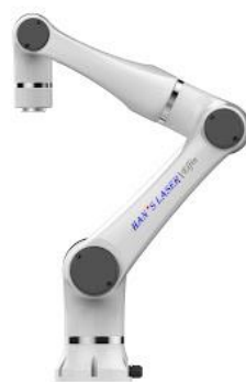
Figure 3.6: The Elfin 5 robot made by Han's Robot.
