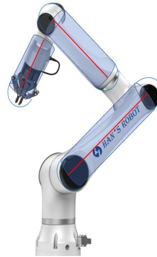
Figure 3.8: SSLs model of the moving links of the Elfin 5 robot
