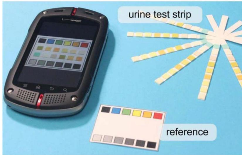
**Figure 2.8** Smartphone analysis of urine test strips [140]. Smartphone images of colorimetric test strips are compared against a reference color chart to detect analytes in urine. (Copyright Permission Granted).
