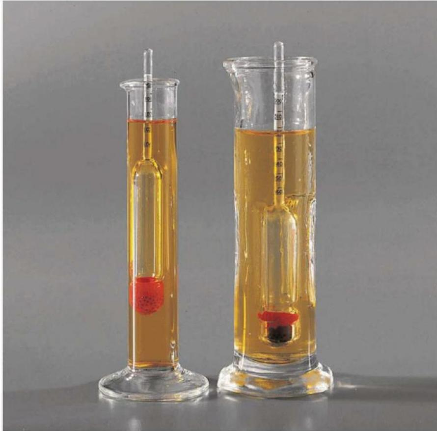
**Figure 2.12** Example of hydrometer for urine specific gravity assessment [142]. (Copyright Permission Granted).
