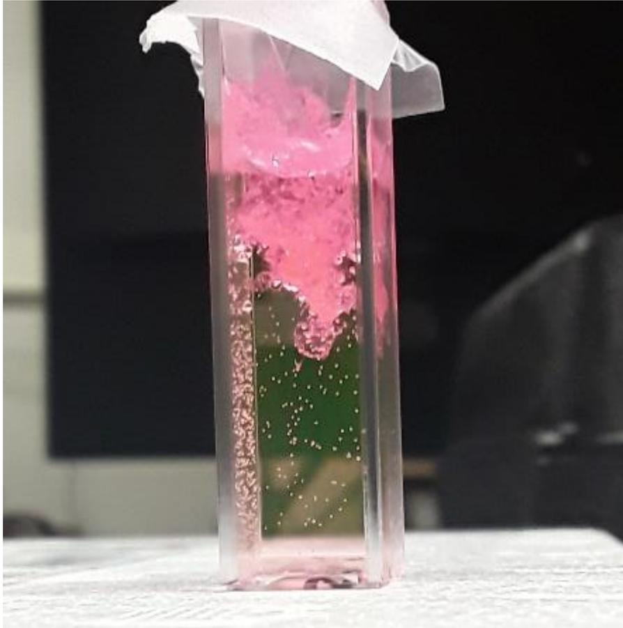
**Figure 5.14** A gelled Eosin dye mixture when directly injected into a cuvette of basic solution ( $\text{pH} > 10.5$ ).
