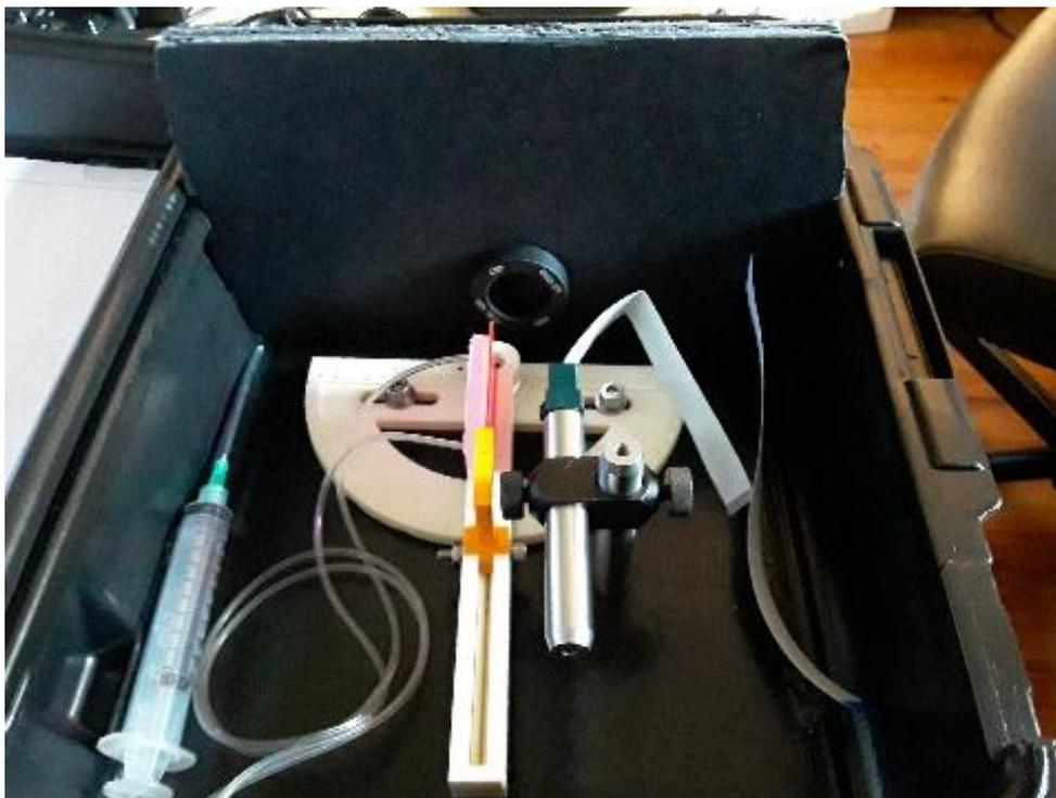
**Figure 5.18** The measurement compartment inside of the portable prototype fluorescence chip reader.
