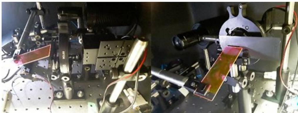
**Figure 5.9** Experimental setup for exciting an Eosin-coated slide from the edge using a 450 nm laser line profile through a slit.
