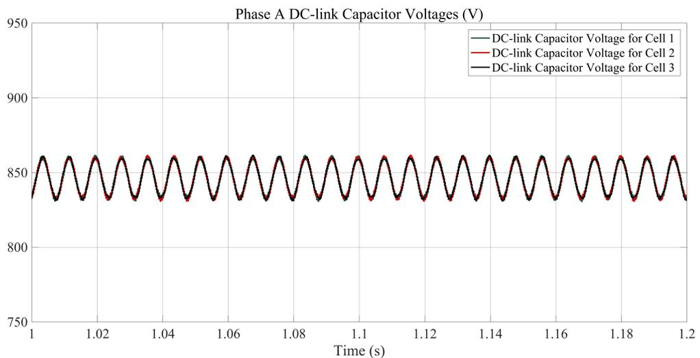
Fig. 2.17 Dc-link capacitor voltages for three non-regen CHB power cells in phase A.
