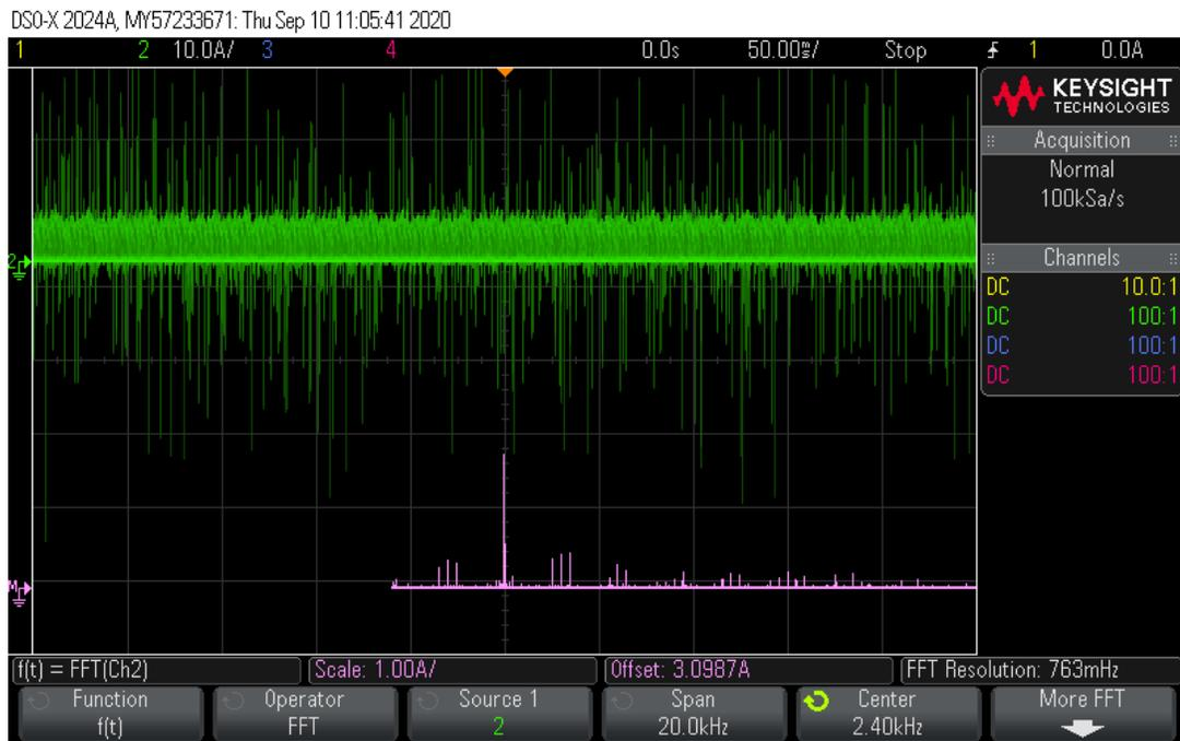
Fig. 7.10 3-phase AFE rectifier dc-bus current and spectrum without CST.
