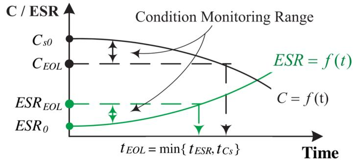
Fig. 3.11 Indicators condition monitoring range [50] and EOL spot determination.
