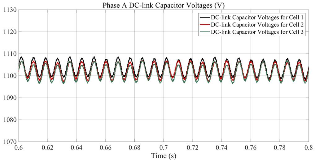
Fig. 2.21 Dc-link capacitor voltages for three regen CHB power cells in phase A.
