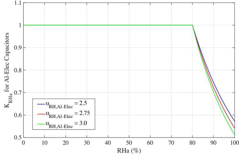
Fig. 4.1.7 Humidity stress factor curves for different  $\alpha_{RH,Al-Elec}$ .
