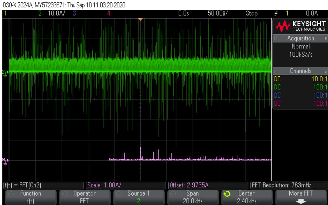
Fig. 7.13 3-phase AFE rectifier dc-bus current and spectrum with CST.
