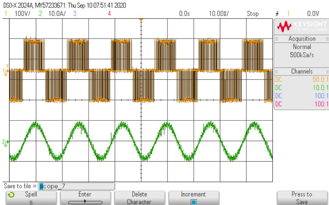
Fig. 7.9 Output voltage and current waveforms of a regen CHB power cell.
