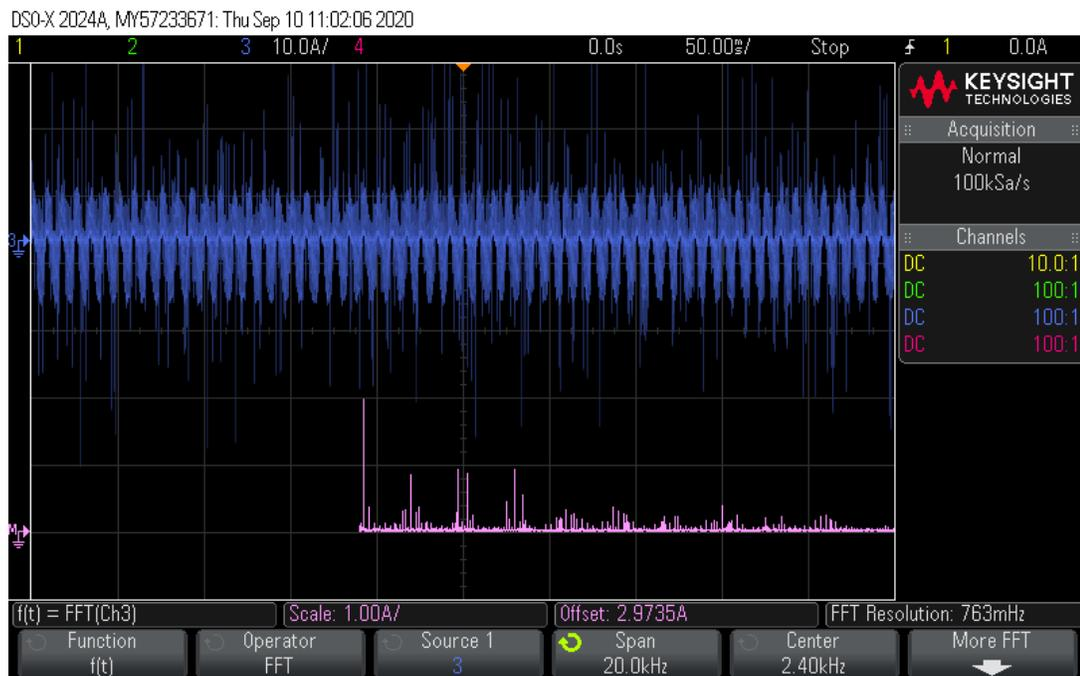
Fig. 7.15 Dc-link capacitor current and spectrum with CST.
