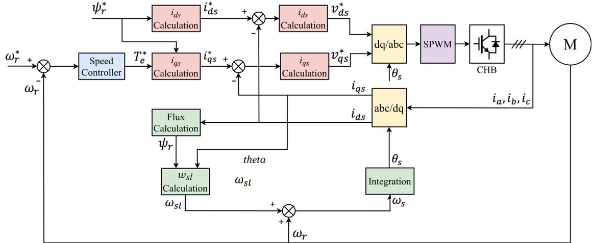
Fig. 2.15 Indirect FOC for rotor flux orientation.
