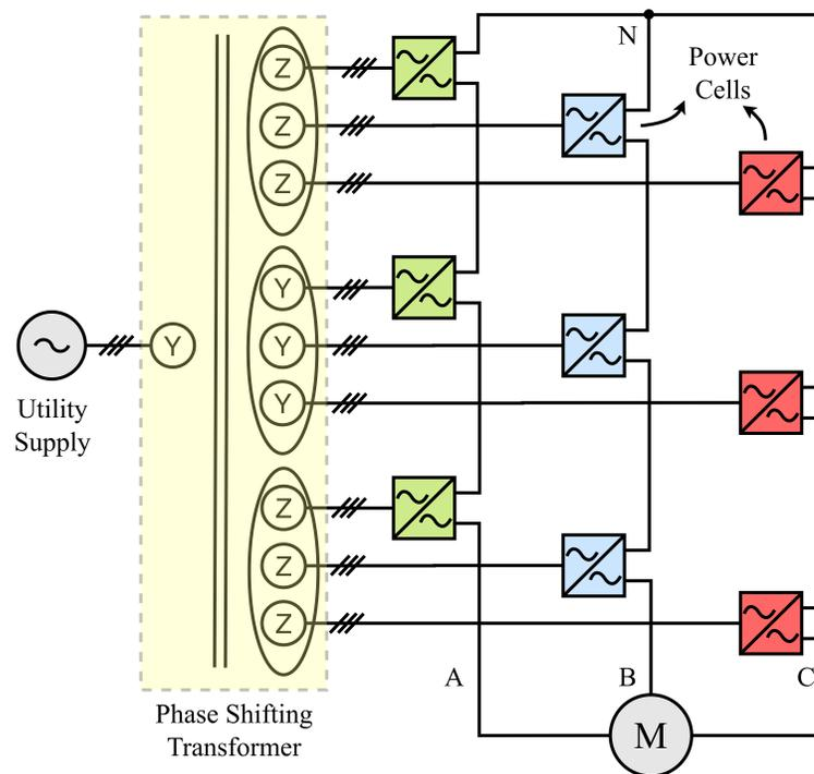
Fig. 2.1. A 3-phase 7-level CHB motor drive.
