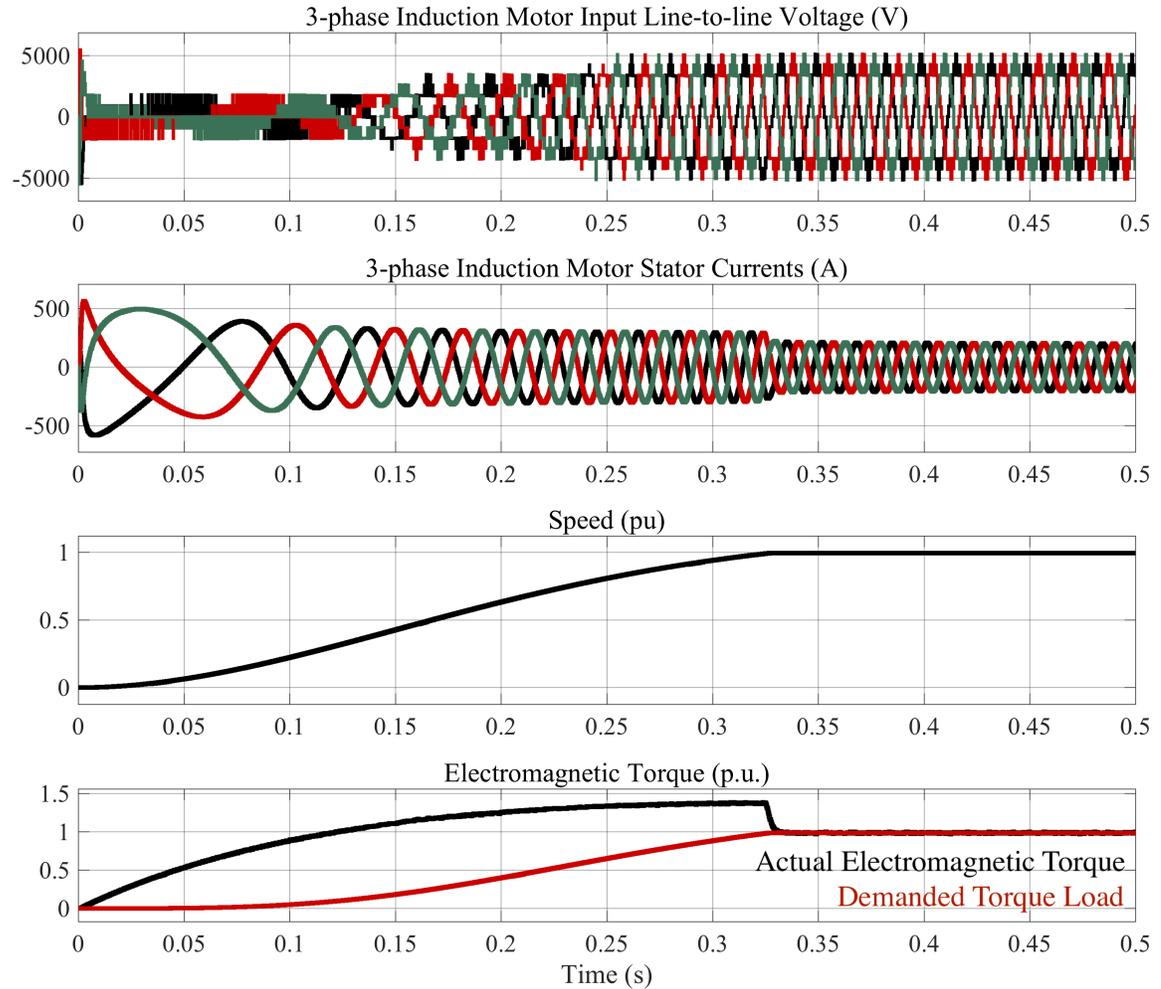
Fig. 2.19 Induction motor waveforms in non-regen condition.
