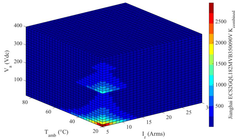
Fig. 4.3.1 4-D image of  $K_{combined}$  for Jianghai ECS2GQL182MVB350090V.
