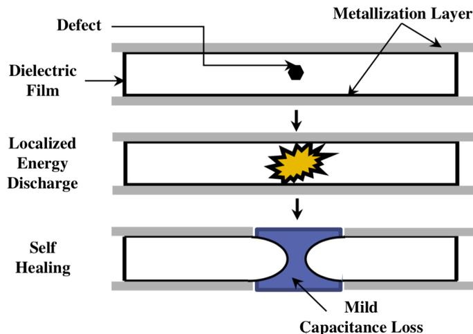
Fig. 3.5 Self-healing process of a metallized film [22].
