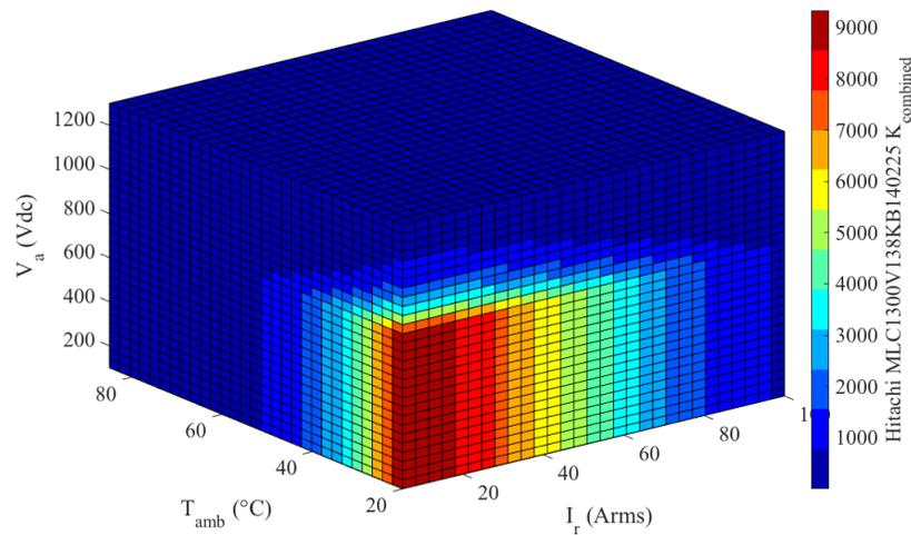
Fig. 4.3.3 4-D image of  $K_{combined}$  for Hitachi MLC1300V138KB140225.
