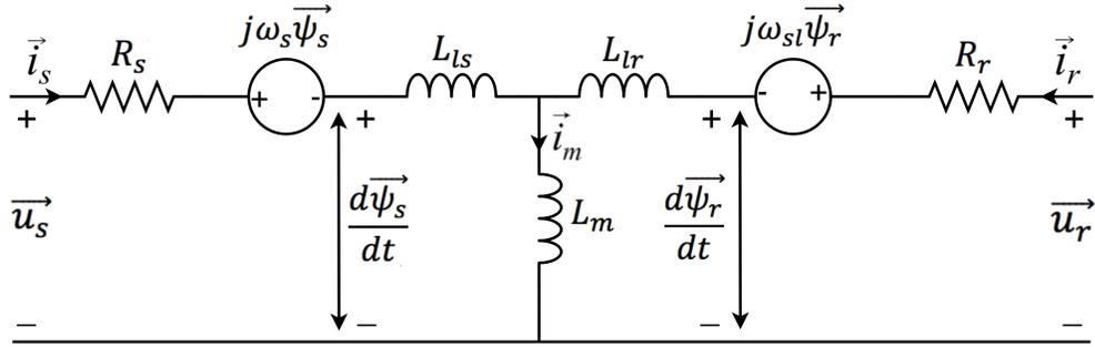
Fig. 2.13 Induction motor circuit.
