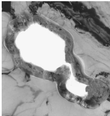
Fig. 3.3 An etched pole on anode foil. Light grey: aluminum. Dark grey:  $\text{Al}_2\text{O}_3$  [15].
