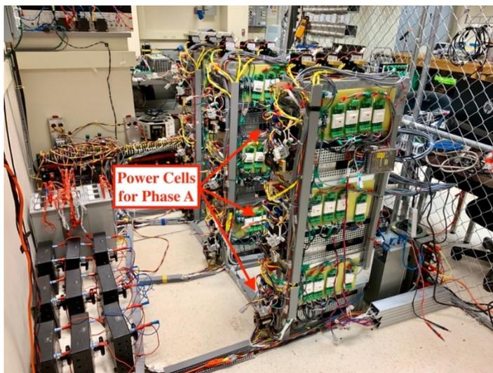
Fig. 7.2 Layout of 3-phase 7-level CHB inverter.
