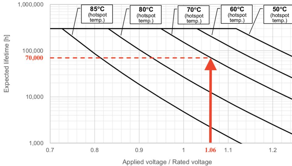
Fig. 4.3.11 Lifetime multiplier location 3) in Hitachi MLC1300V138KB140225's MLD.
