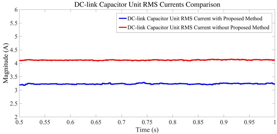
Fig. 6.9 Dc-link general rms currents comparison of Jianghai Al-Elec capacitor unit.
