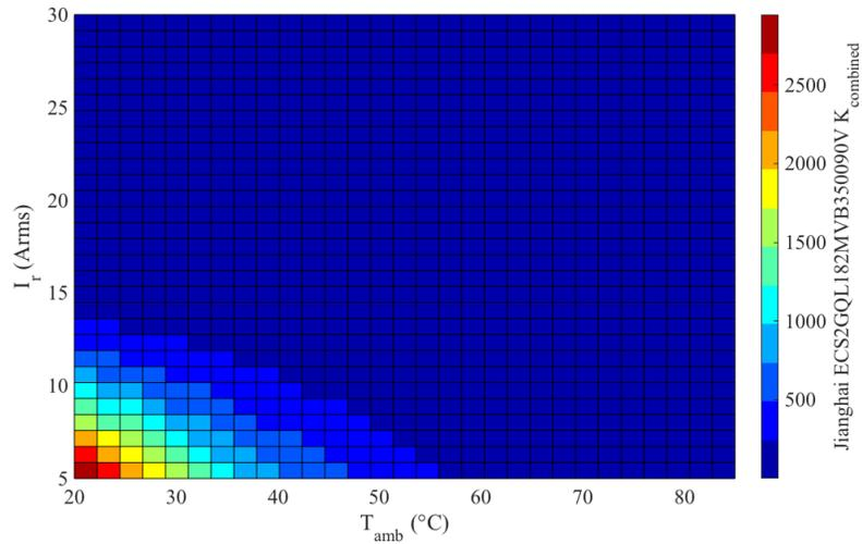
(a)  $I_r - T_{amb}$  view.
