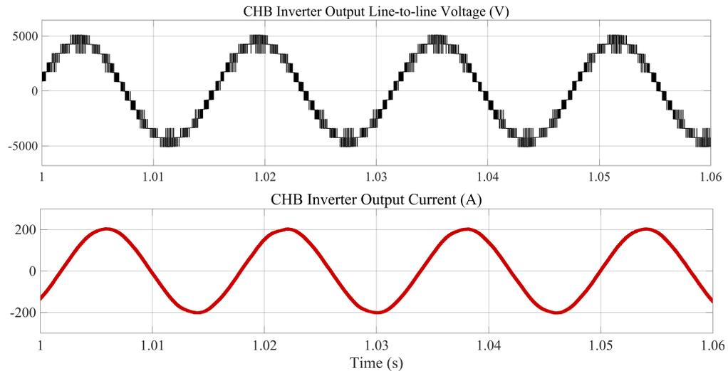
Fig. 2.16 Non-regen CHB inverter output line-to-line voltage and output current.
