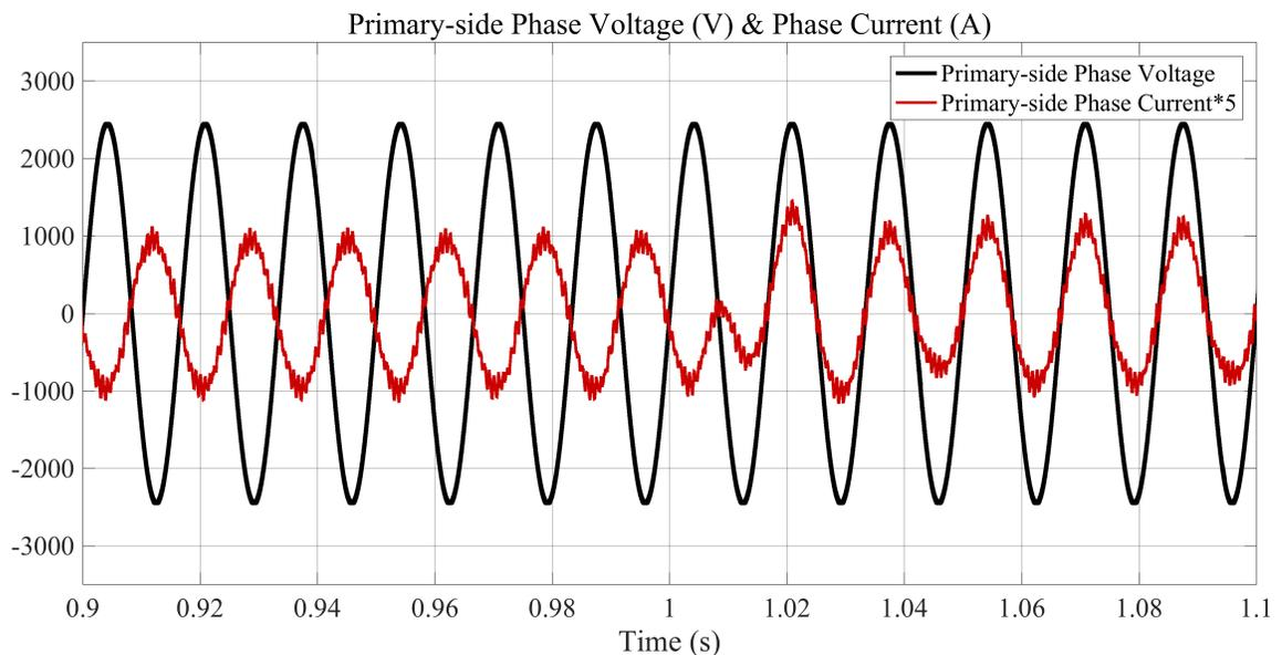
Fig. 2.22 Primary-side phase voltage and phase current of phase-shifting transformer in regen condition.
