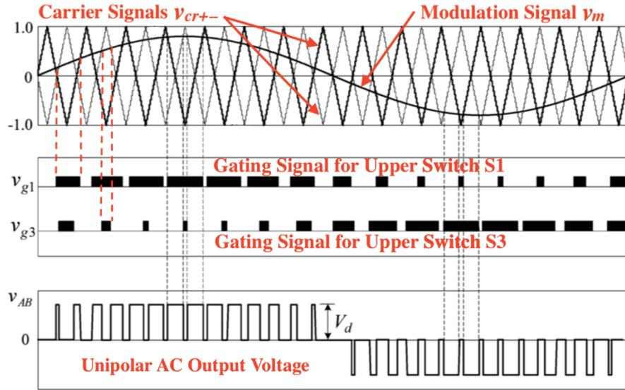
Fig. 2.3 SPWM pattern for a single-phase H-Bridge inverter [7].
