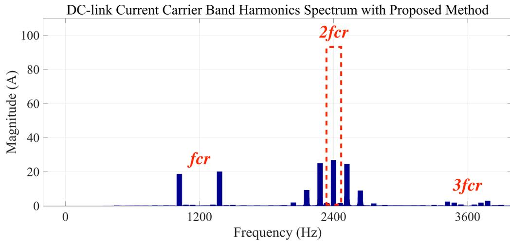
Fig. 5.9 Dc-link capacitor current carrier band harmonics spectrum with CST.
