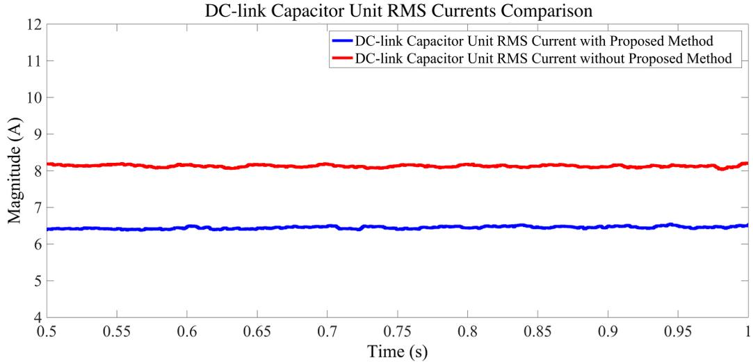
Fig. 6.12 Dc-link general rms currents comparison of Hitachi MPPF capacitor unit.
