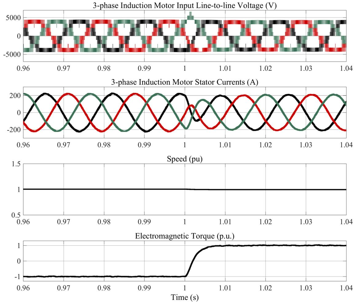
Fig. 2.23 Induction motor waveforms in regen condition.
