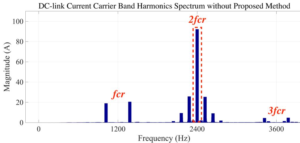
Fig. 5.8 Dc-link capacitor current carrier band harmonics spectrum without CST.
