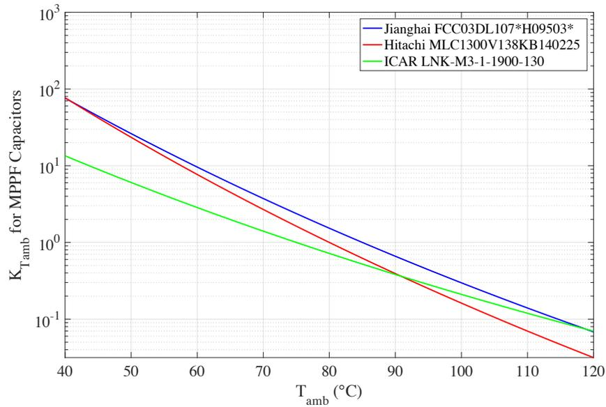
Fig. 4.1.4 Ambient temperature stress factor curves for 3 MPPF power capacitors.
