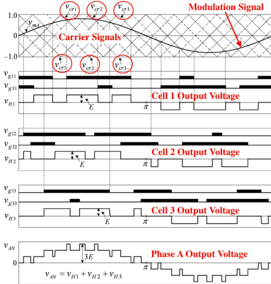
Fig. 2.5 SPWM pattern of a phase leg of 7-level CHB inverter [7].
