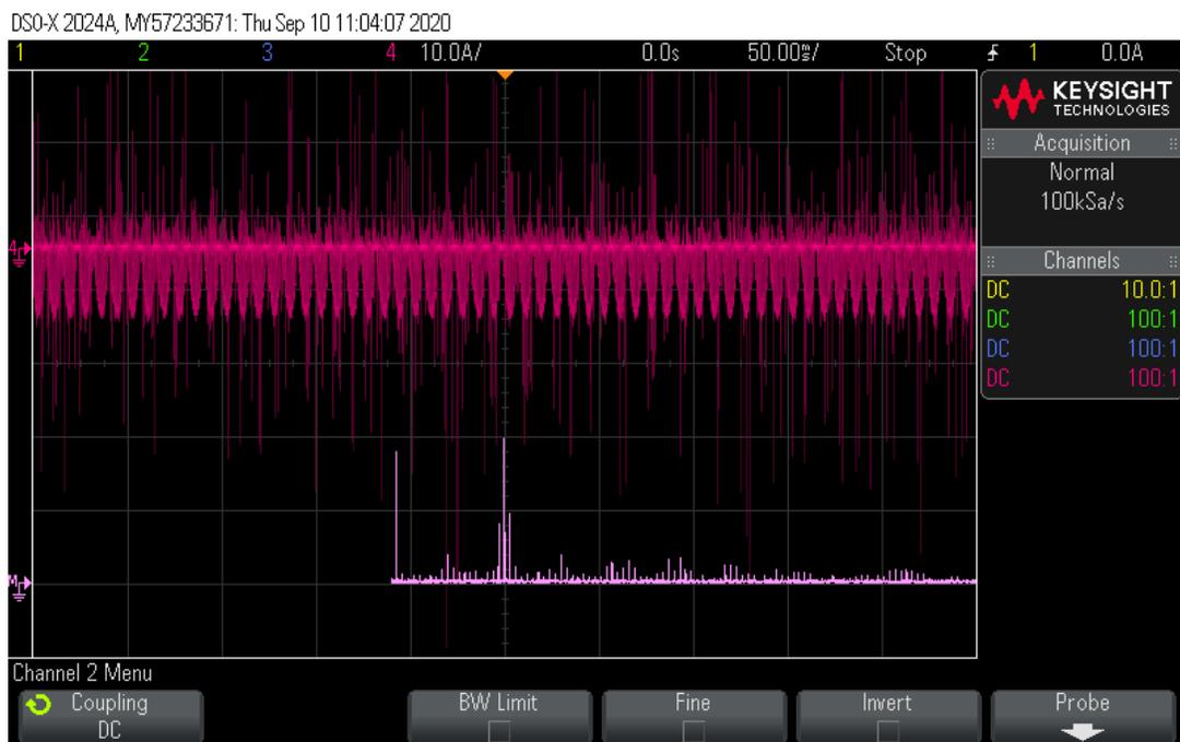
Fig. 7.11 H-bridge inverter dc-bus current and spectrum without CST.
