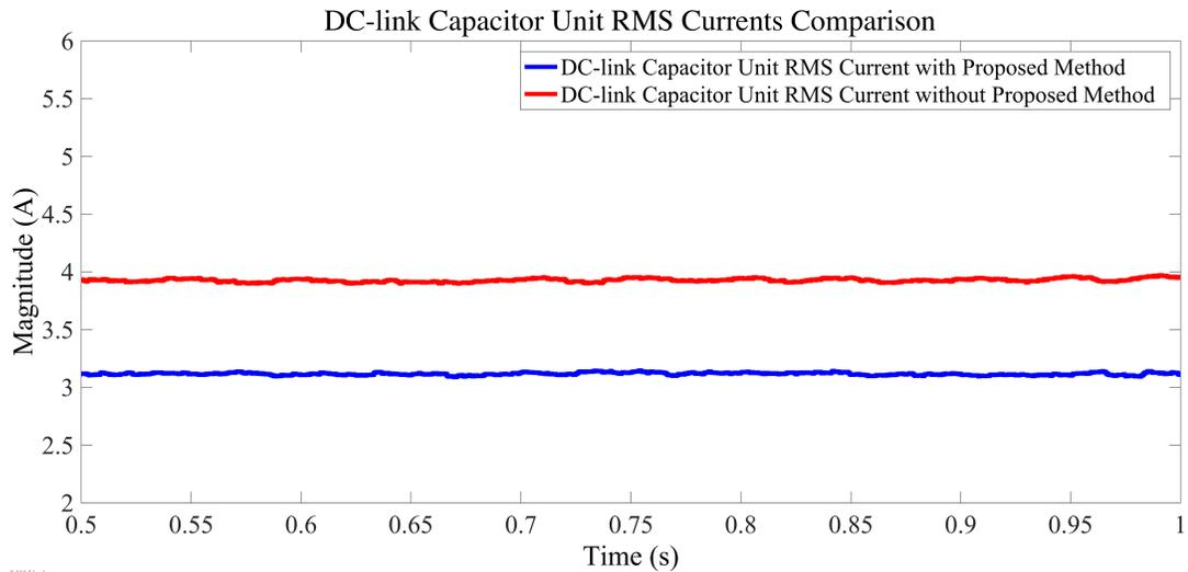
Fig. 6.10 Dc-link general rms currents comparison of Hitachi Al-Elec capacitor unit.
