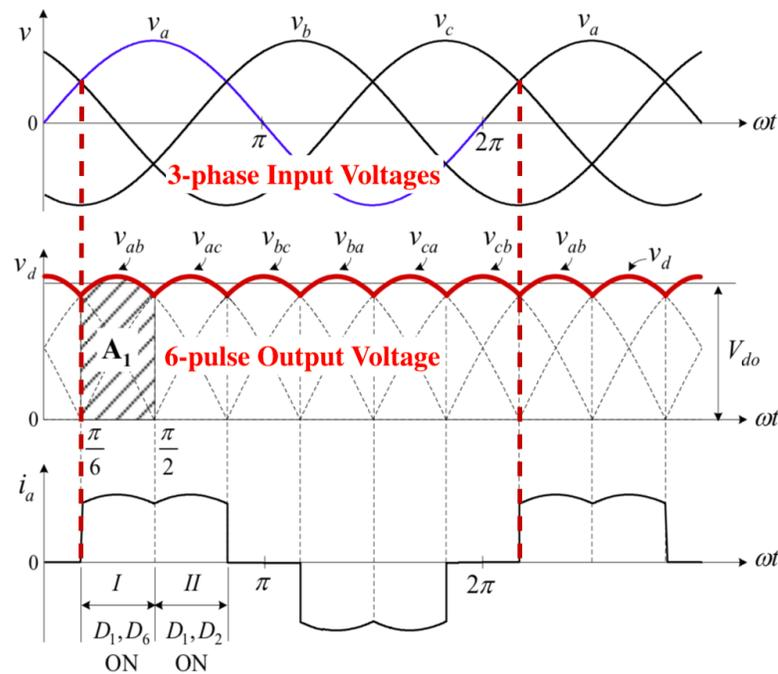
Fig. 2.7 Conducting states of 3-phase 6-pulse DFE rectifier [9].
