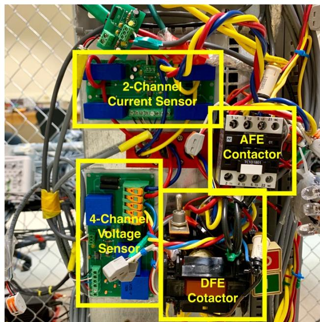
Fig. 7.6 Sensors and contactors.
