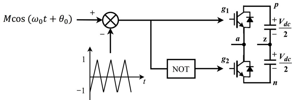
Fig. 5.2 SPWM scheme for one converter phase leg.
