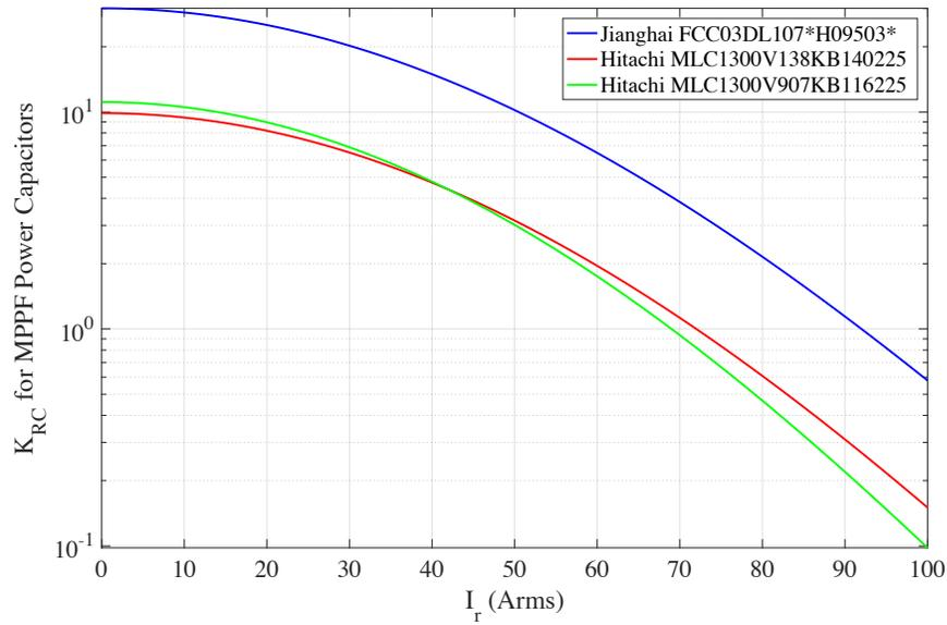
Fig. 4.1.2 Ripple current stress factor curves for 3 MPPF power capacitors.
