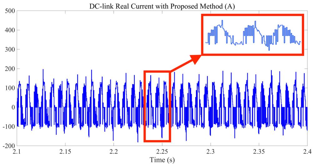
Fig. 5.12 Dc-link capacitor real current with CST.
