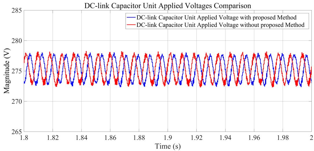
Fig. 6.2 Dc-link applied voltages of Jianghai Al-Elec capacitor unit.
