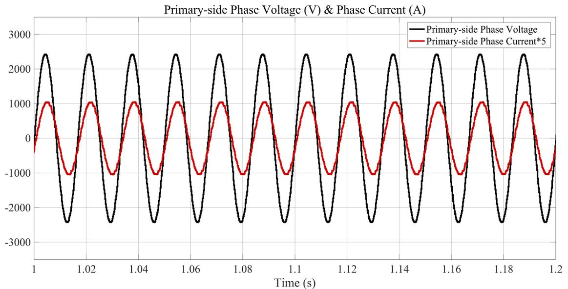
Fig. 2.18 Primary-side phase voltage and phase current of phase-shifting transformer in non-regen condition.
