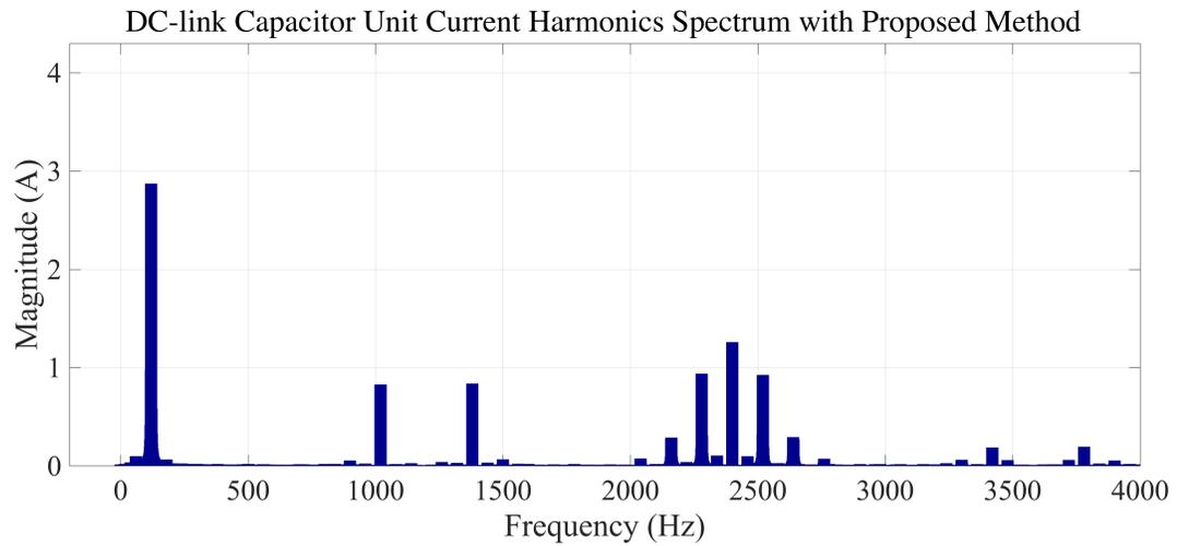
Fig. 6.1 Dc-link current harmonics spectrums of Jianghai Al-Elec capacitor unit.
