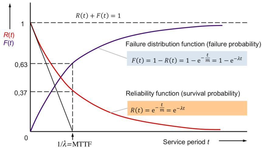
Fig. 4.2.2 MTTF, failure and reliability function with exponential form [67].
