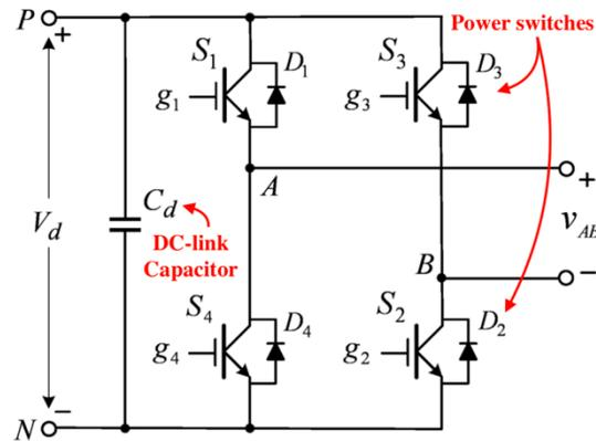
Fig. 2.2 A single-phase H-Bridge inverter [7].
