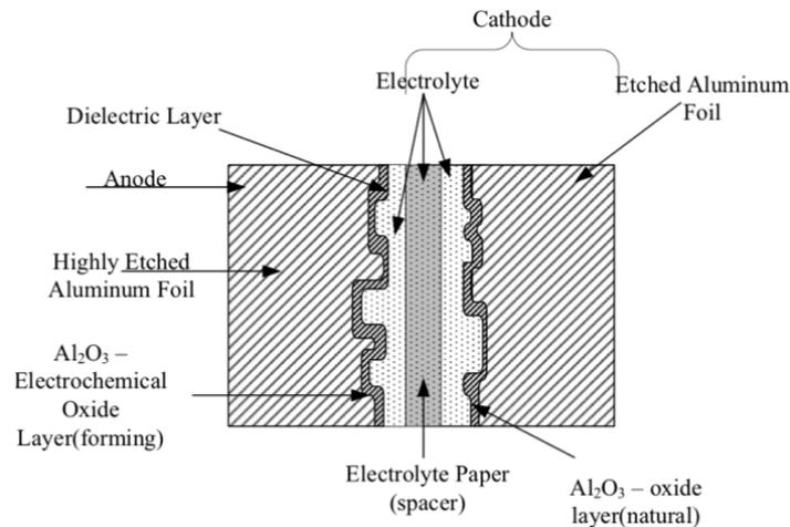
Fig. 3.1 Structure of an aluminum electrolytic capacitor [11].
