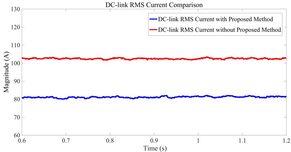
Fig. 5.13 Dc-link capacitor rms current with/without CST.
