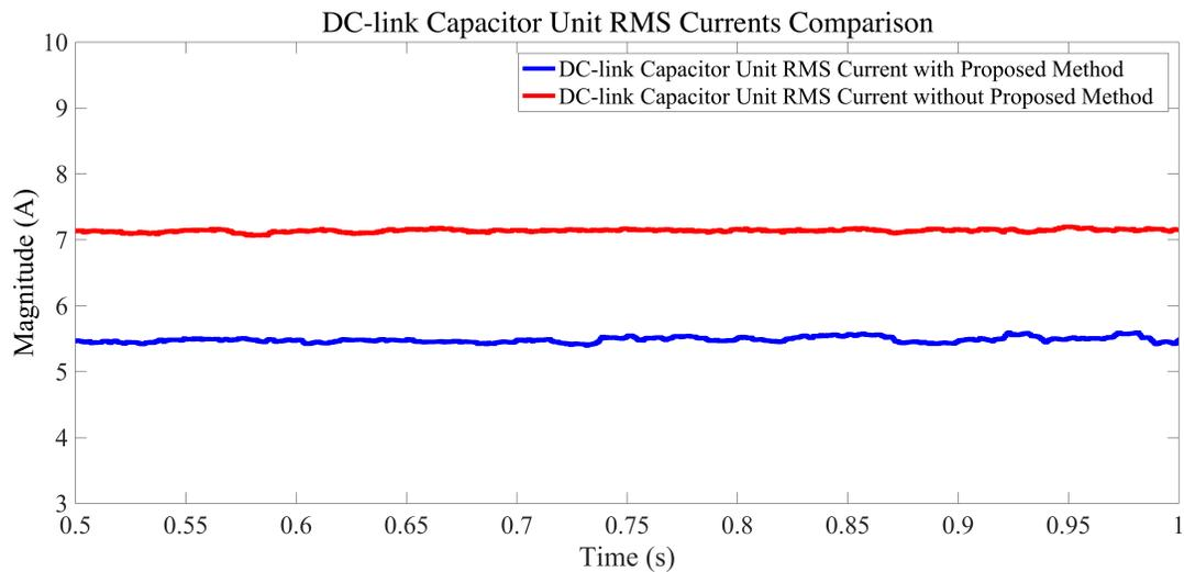
Fig. 6.11 Dc-link general rms currents comparison of Jianghai MPPF capacitor unit.
