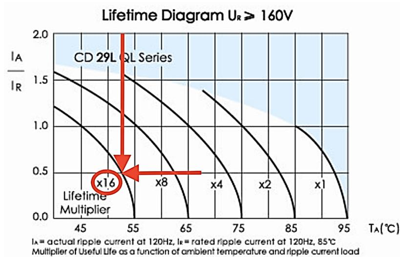
Fig. 4.3.6 Lifetime multiplier location 2) in Jianghai ECS2GQL182MVB350090V's
