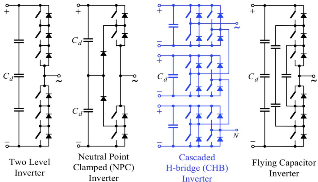
Fig. 1.1 Per phase topologies of typical multilevel inverters [3].
