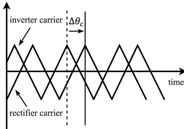
Fig. 5.4 Definition of carrier shifted angle  $\Delta\theta_c$ .
