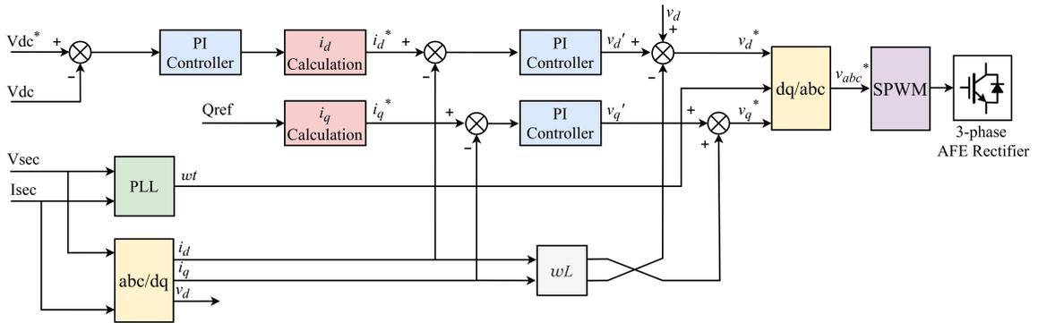
Fig. 2.9 3-phase AFE rectifier controller.
