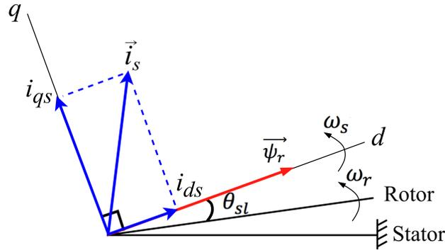
Fig. 2.14 Rotor flux orientation.
