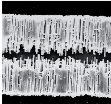
Fig. 3.2 An etched foil for high voltage anode [14].
