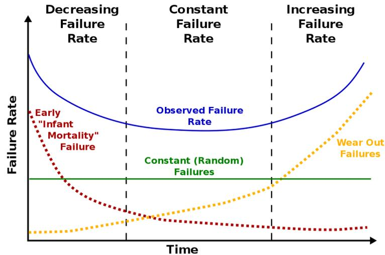
Fig. 4.2.1 Bathtub curve with three failure rate sections [68].
