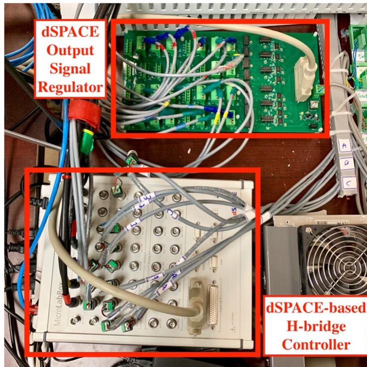
Fig. 7.8 dSpace-based H-bridge inverter control platform.
