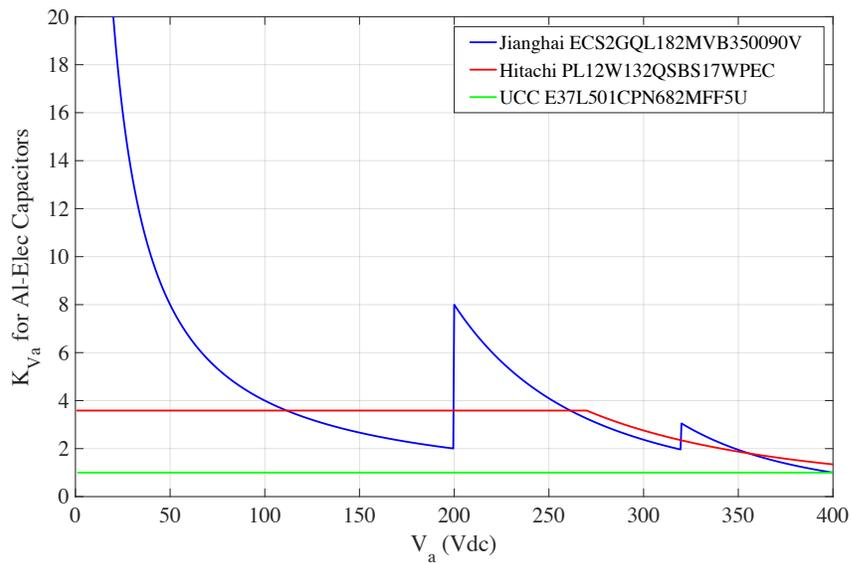
Fig. 4.1.5 Applied voltage stress factor curves for 3 Al-Elec power capacitors.
