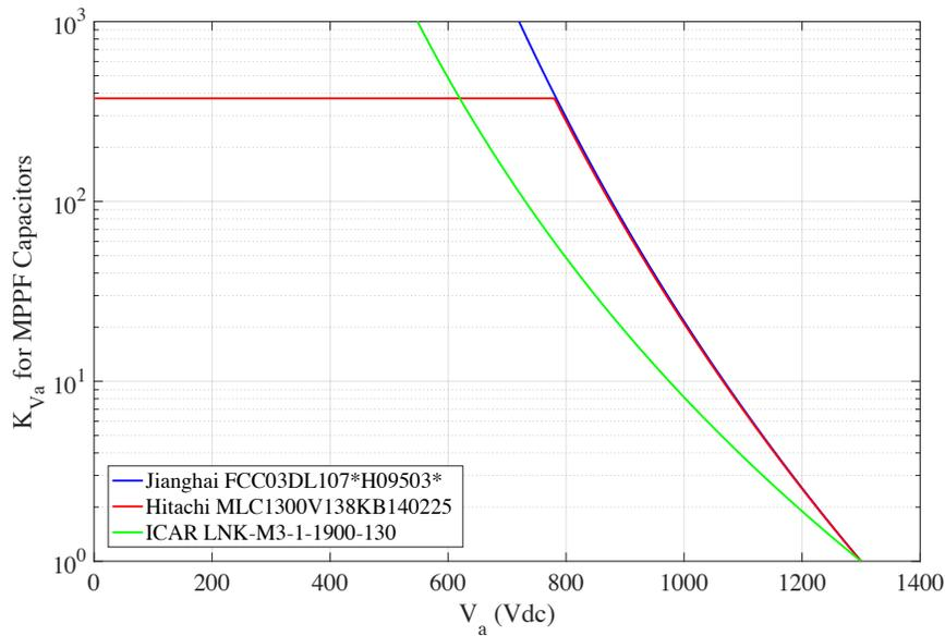
Fig. 4.1.6 Applied voltage stress factor curves for 3 MPPF power capacitors.
