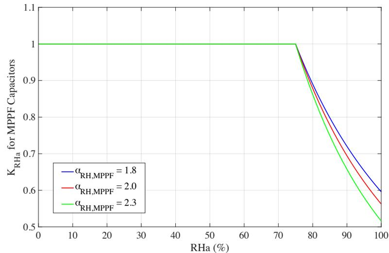
Fig. 4.1.8 Humidity stress factor curves for different  $\alpha_{RH,MPPF}$ .
