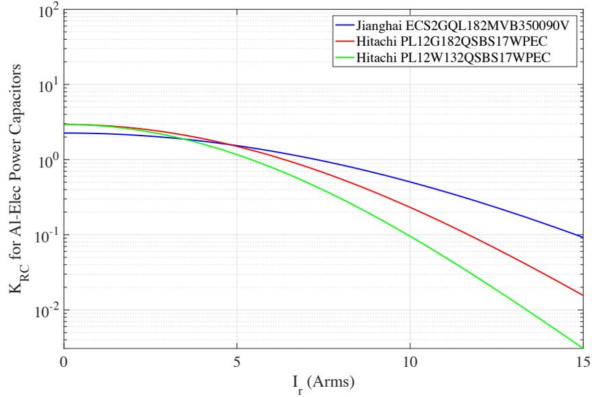
Fig. 4.1.1 Ripple current stress factor curves for 3 Al-Elec power capacitors.
