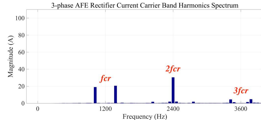
Fig. 5.6 3-phase AFE rectifier current carrier band harmonics spectrum.
