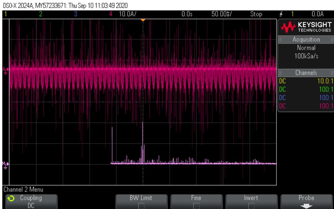
Fig. 7.14 H-bridge inverter dc-bus current and spectrum with CST.
