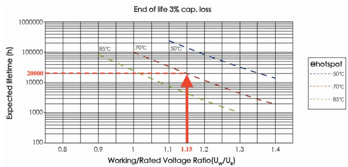
Fig. 4.3.9 Lifetime multiplier location 1) in Jianghai FCCC3DL107\*H09503\*'s MLD.
