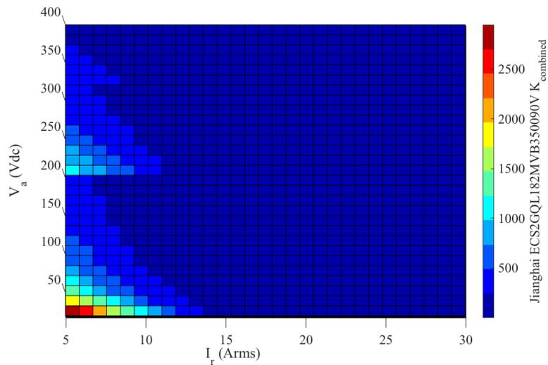
(b)  $I_r - V_a$  view.Fig. 4.3.2 Different views of  $K_{combined}$  for Jianghai ECS2GQL182MVB350090V.
