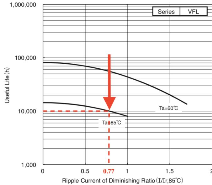
Fig. 4.3.8 Lifetime multiplier location 4) in Hitachi VFL2G103YQE188's MLD.
