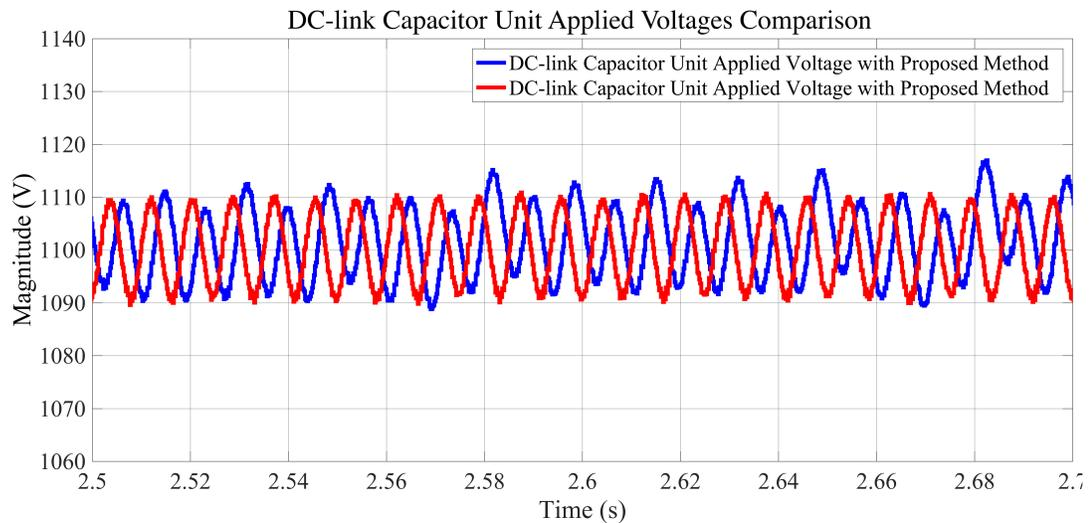
Fig. 6.6 Dc-link applied voltages of Jianghai MPPF capacitor unit.
