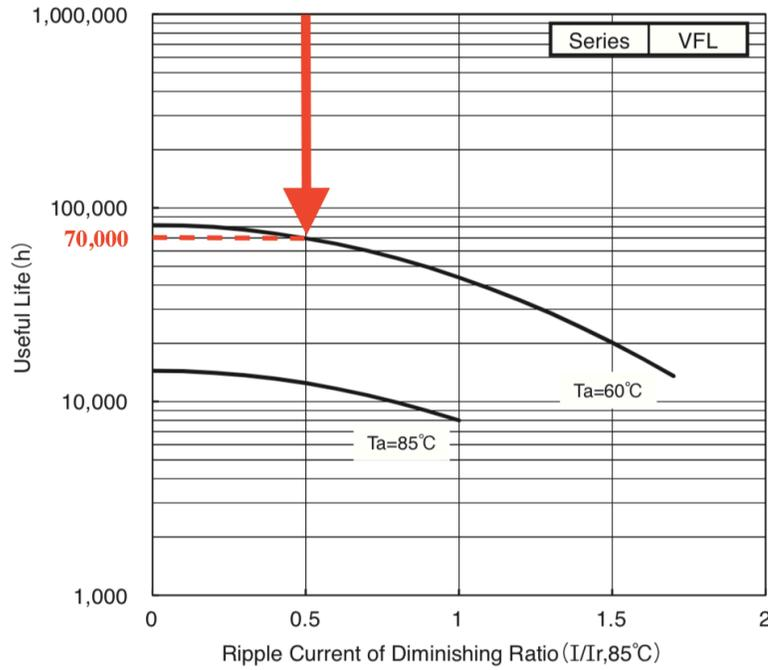
Fig. 4.3.7 Lifetime multiplier location 3) in Hitachi VFL2G103YQE188's MLD.
