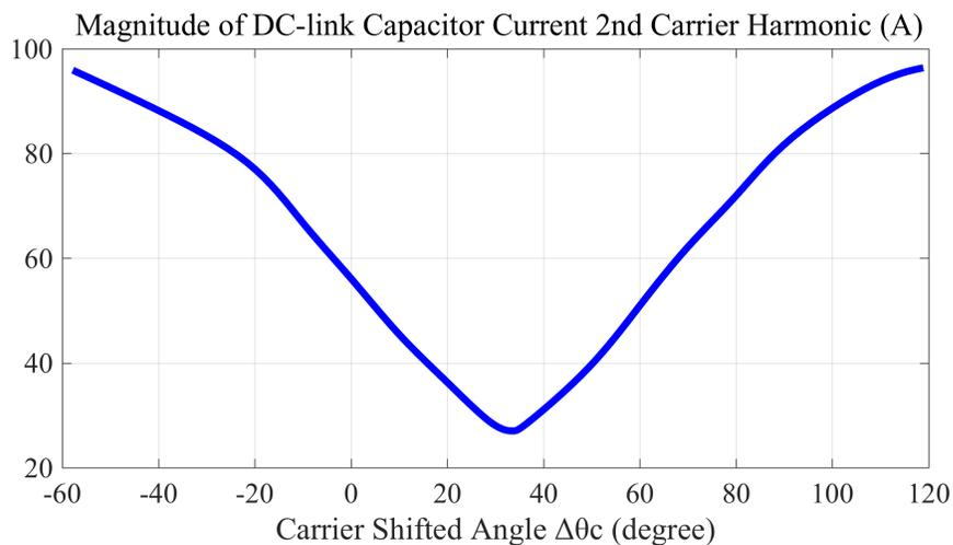
Fig. 5.10 Magnitude of 2<sup>nd</sup> central carrier harmonic vs. carrier shifted angle.
