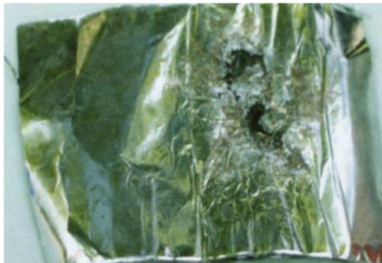
Fig. 3.6 Intense self-healing causes film explosion [23].
