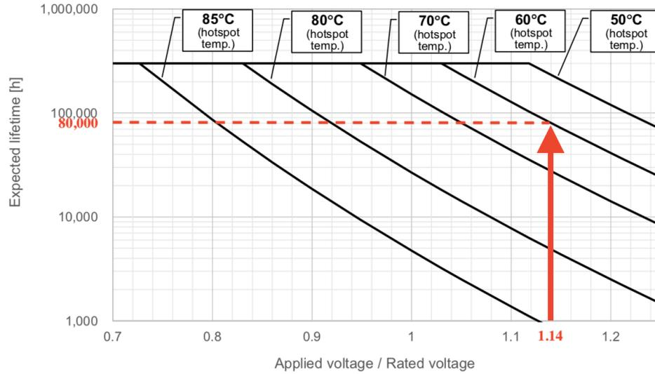
Fig. 4.3.12 Lifetime multiplier location 4) in Hitachi MLC1300V138KB140225's MLD.
