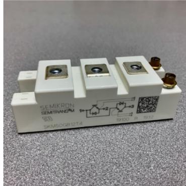
Fig. 7.4 Half-bridge IGBT module.
