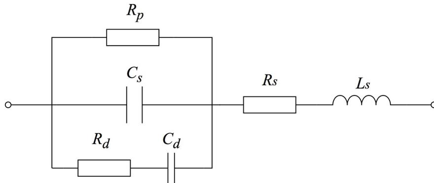
Fig. 3.9 Ubiquitous circuit model for dc-link power capacitors.
