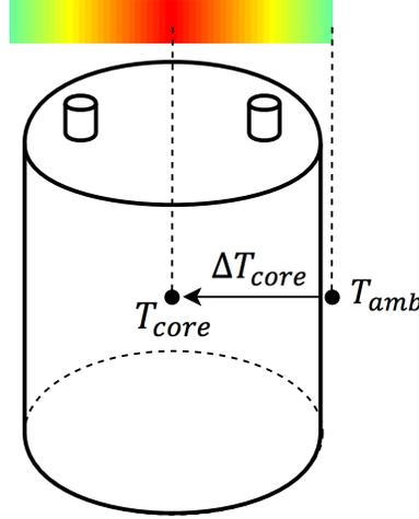
Fig. 3.7 Definition of a capacitor's core temperature.
