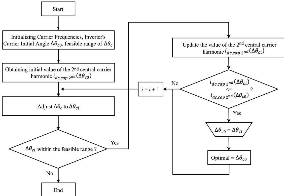
Fig. 5.5 Flowchart of proposed CST with optimization ideology.
