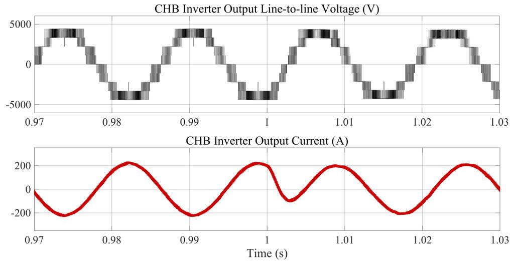
Fig. 2.20 Regen CHB inverter output line-to-line voltage and output current.
