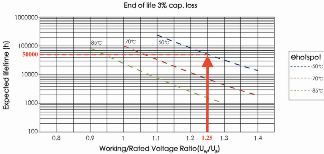
Fig. 4.3.10 Lifetime multiplier location 2) in Jianghai FCCC3DL107\*H09503\*'s MLD.
