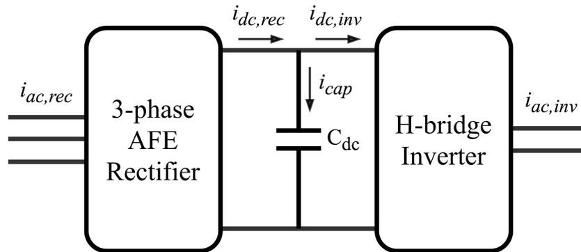
Fig. 5.1 Current flow of a regen CHB power cell.
