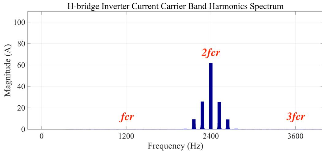
Fig. 5.7 H-bridge inverter current carrier band harmonics spectrum.
