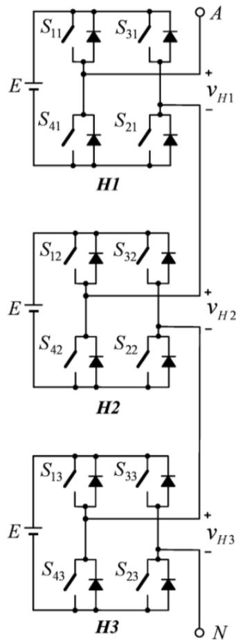
Fig. 2.4 A phase leg of 7-level CHB inverter [7]: 3 single-phase H-bridge inverter are cascaded in series.
