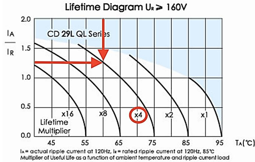
Fig. 4.3.5 Lifetime multiplier location 1) in Jianghai ECS2GQL182MVB350090V's
