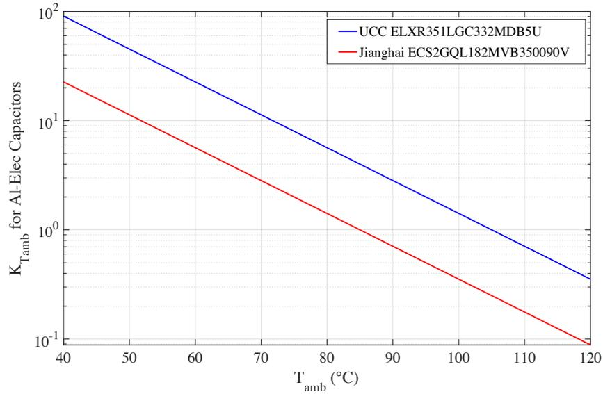
Fig. 4.1.3 Ambient temperature stress factor curves for 2 Al-Elec power capacitors.
