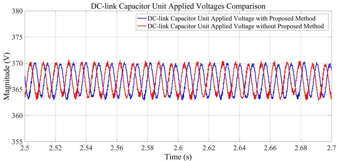
Fig. 6.4 Dc-link applied voltages of Hitachi Al-Elec capacitor unit.
