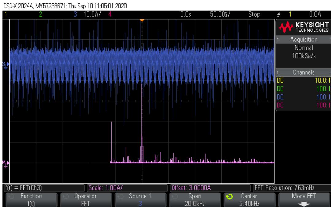
Fig. 7.12 Dc-link capacitor current and spectrum without CST.
