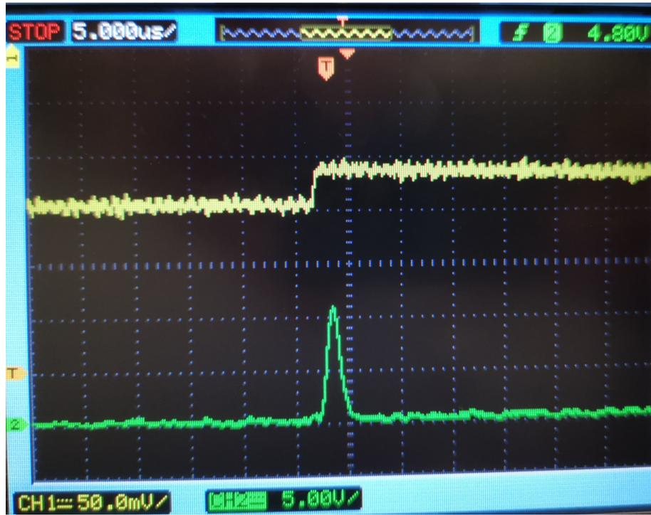
Figure 6.2: Preamp output (CH1, yellow) and shaping amp output signal (CH2, green) of the ScCVDD detector at 60 V. 5X amplitude magnification on oscilloscope display
