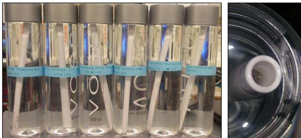
**Figure 6.** Pictures of single channel tubular ceramic membranes stored in DI water. Note that a total of 6 ceramic membranes are shown in the picture but only 4 of them were used for wastewater filtration studies in this report. Panel on the right shows the hollow feed channel inside the tubular membrane which contains the membrane active surface. Each membrane was 25 cm in length with an active membrane area of 55 cm<sup>2</sup>
