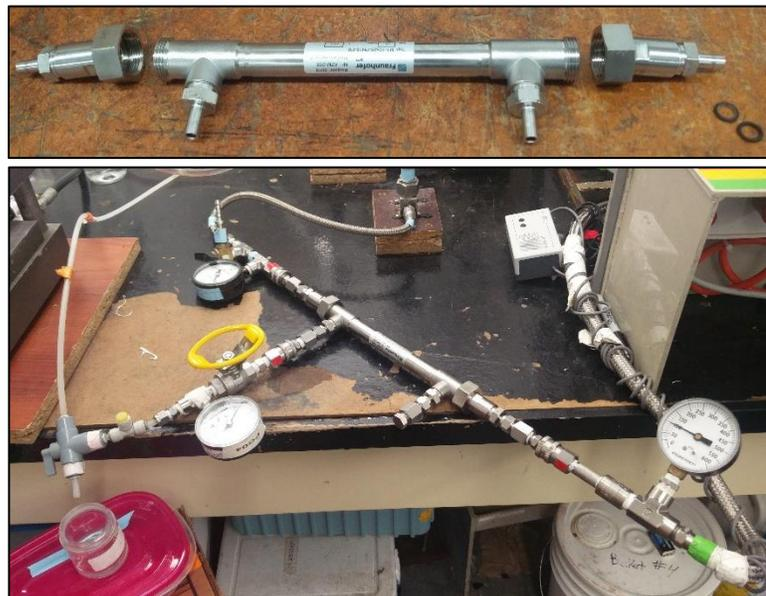
**Figure 11.** Pictures of the ceramic membrane testing module. Top panel shows the module with ends detached and o-rings placed on the side. Bottom panel shows the module attached to the setup and in operation. Note that the membrane had two permeate outlets (top panel) one of which was blocked (bottom panel) to redirect all permeate from only one outlet.
