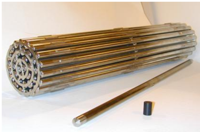
Figure 2. CANDU Fuel Bundle Photograph: Assembled Bundle, Single Fuel Element, and Single Fuel Pellet [11]
