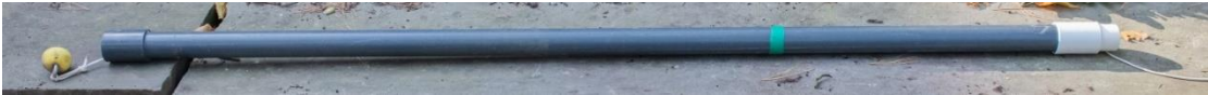
Figure 2.6: Septic tank sampling apparatus. A.) Effluent sampler (top) – A PVC container with an approximate volume of 0.75 L attached to the bottom of a ~4 ft. pole with two metallic screws. Collection vessel (bottom) – A PVC container with an approximate volume of 1.25 L attached to the bottom of a ~4 ft. plastic pole with two metallic screws. B.) Tube sampler – A ~4 ft. hollow plastic tube with two open ends. A rope with a hard foam ball on the bottom end (left) runs through the entire length of the tube and exits at the white-tipped end at the top of the tube (right). A screw protrudes near the top of the tube below the white-tipped end to serve as a hook for the rope to be secured on. The green tape designates an approximate 1 L volume mark of the sampler.
