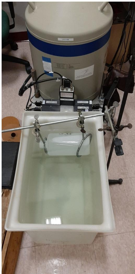
Figure 2.2: Human torso phantom with the liver phantom lowered into the cavity, making it the ideal experimental set-up.
