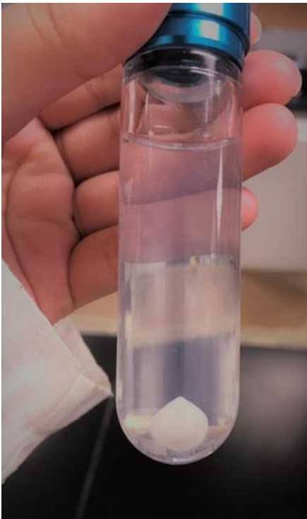
Figure 16: Batch 1: PLGA (3:2) after ultracentrifugation at 12000 rpm for 20 minutes at 24° C
