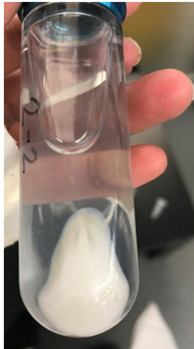
Figure 17: Batch 2: PLGA (50:50) after ultracentrifugation at 10000 rpm for 15 minutes at 24° C
