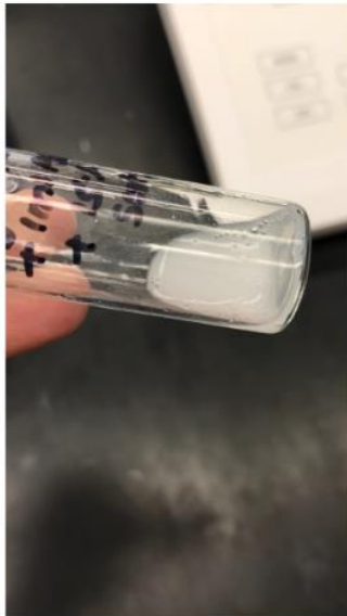
15% PNIPAAm polymer immobilized on PLGA Nanoparticles at Room Temperature
