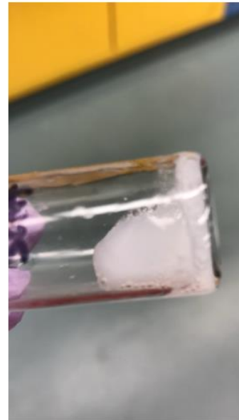
15% PNIPAAm Polymer immobilized on PLGA Nanoparticles at 37°C
