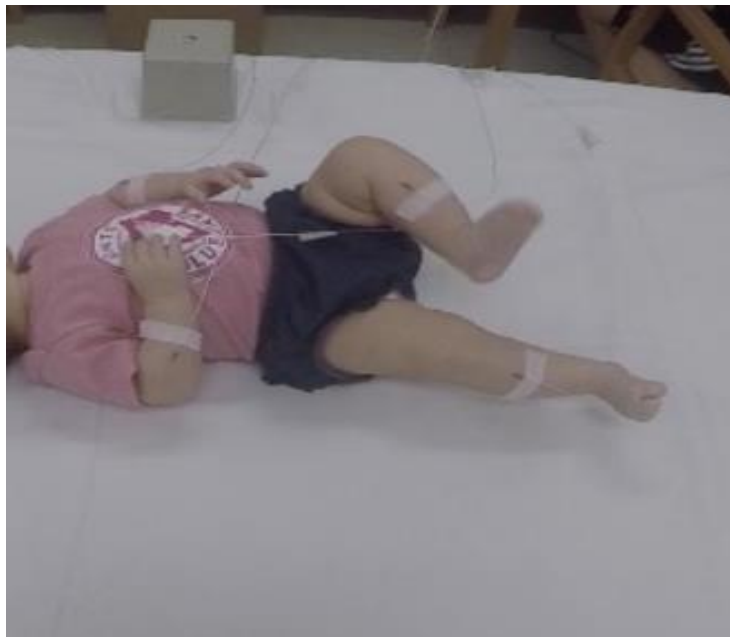
Figure 3.1 Experimental setup of infant GM data collection. The infant is laid on their back and allowed to freely move their limbs while their movements are recorded. The white tapes on the legs and arms are the sensors attached.
