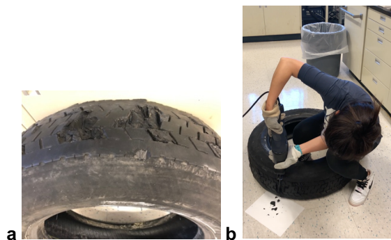
Figure S4.3 (a) Sailun Truck tread 2. (b) Sectioning the external, road contacting section with a reciprocating saw to give Truck tread 2.
