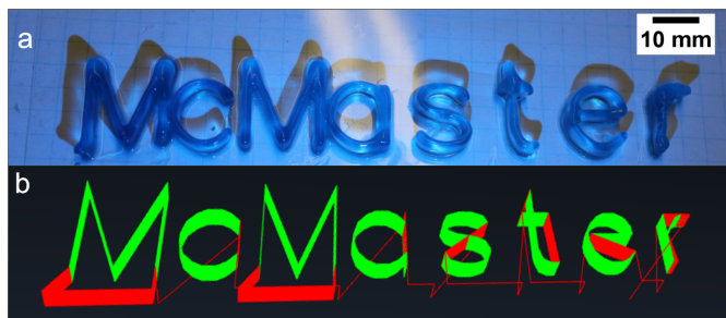
Figure 2.22 (a) The ‘McMaster’ sign printed in silicone elastomer. (b) The gcode illustration; printing moves are in green, while rapid non-printing moves are in red. The rapid moves are absent from the resulting print.
