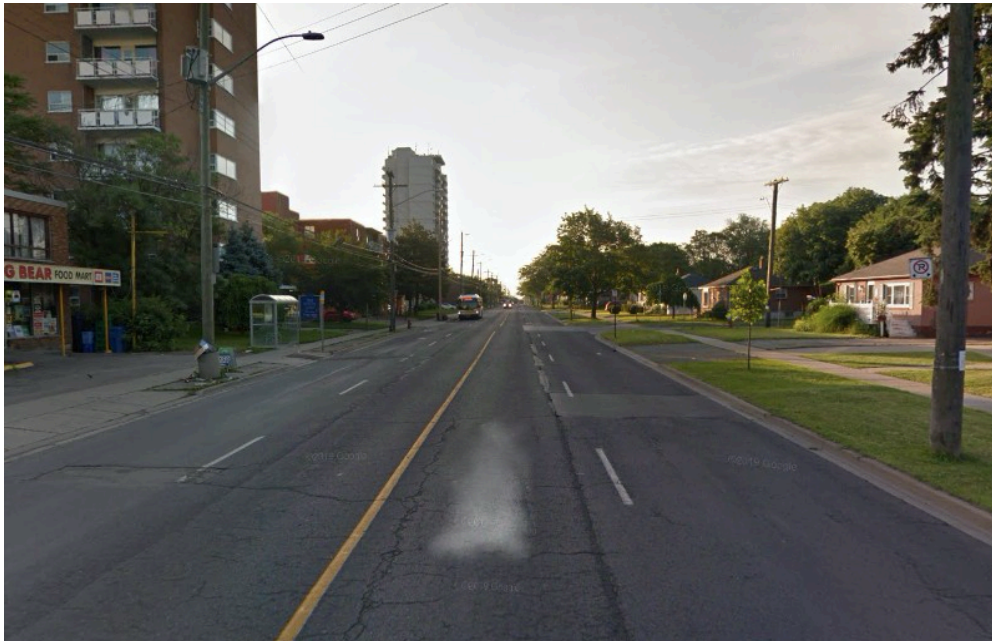
Figure 22. Segment 20 on Route 2B depicting a two-lane arterial road with no on-street parking and a wide grassy verge on the right side of the roadway (Source: Google Street View).
