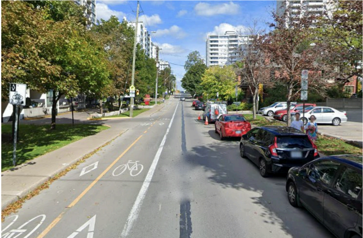
Figure 30. Segment 8 on route 3B depicting a two-way cycle track on a one-way arterial road (Source: Google Street View).
