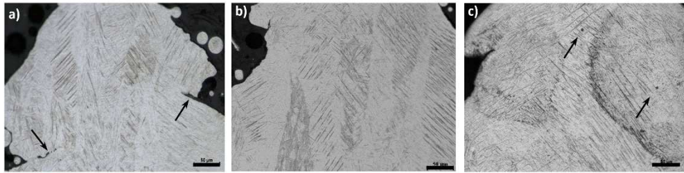
Figure 5-3: Microstructural analysis (a) L-PGGs-3- VED = 42.735 J/mm 3 lack of fusion indicated by arrow, (b) L-PGGs 6- VED= 85.47 J/mm 3 , and (c) L-PGGs 7- VED=192.31 J/mm 3 internal porosities indicated by arrows , scale bar is 50 \mu m.
