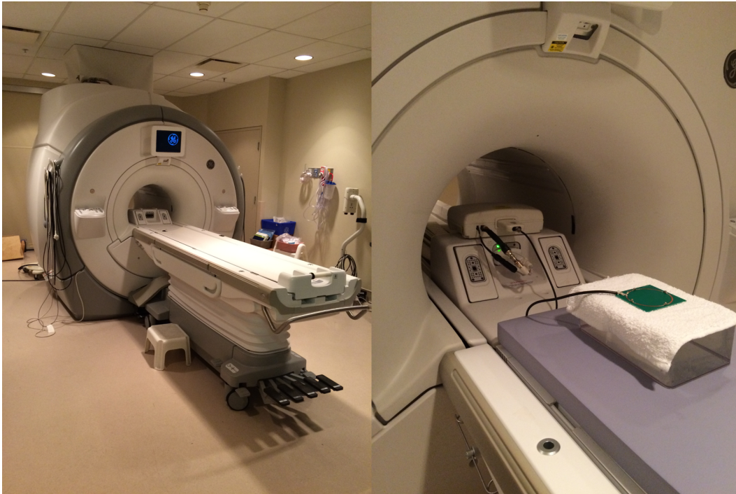
Figure 4.9: MRI Experimental Setup The GE MR730 3T scanner with the circular surface coil connected to the MRI via the sodium T/R switch. The coil can be seen on top of the homogeneity phantom which is covered by a cloth. The phantom itself sits atop a foam riser which centers the coil in the isocentre of the magnet.
