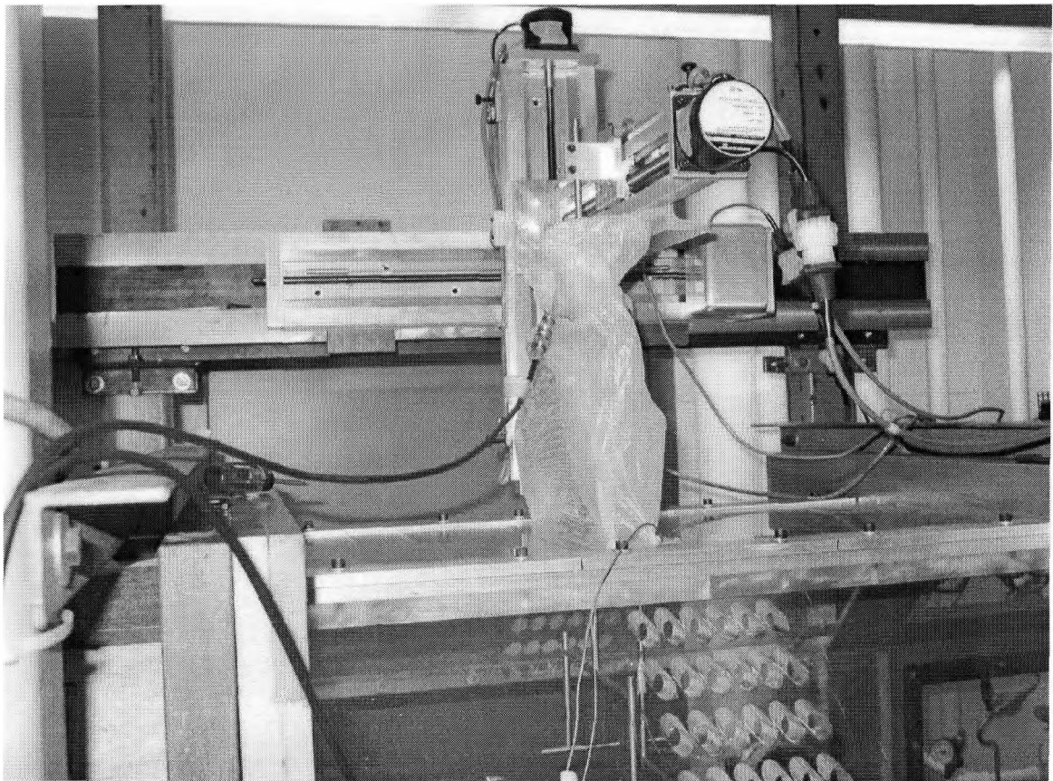
Figure 3.8: Traversing mechanism position above the test section.
