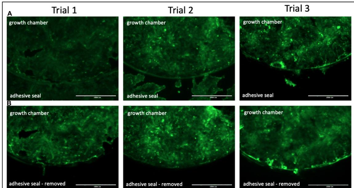
**Figure 7: Maintenance of Calu-3 cellular growth in the targeted growth chamber of an adhesive assembled perfusion chip following adhesive seal removal.**
