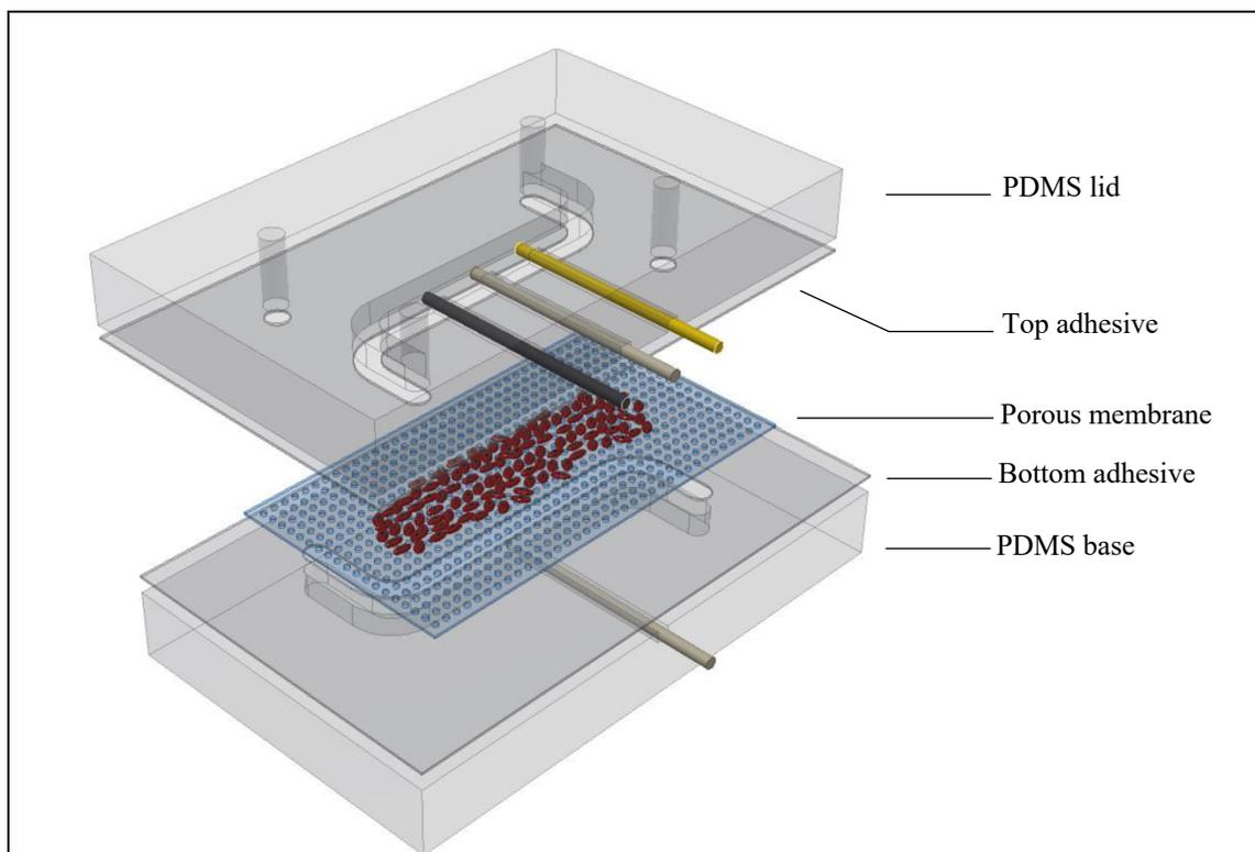
**Figure 11 – Schematic explosion diagram of a rendered adhesive based ALI perfusion chip.**
