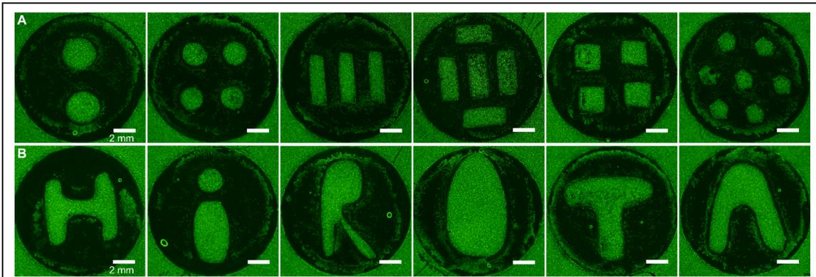
**Figure 4: Xurography cell patterning of HBEC6-KT cells using ARclean® 90716 adhesive.**
