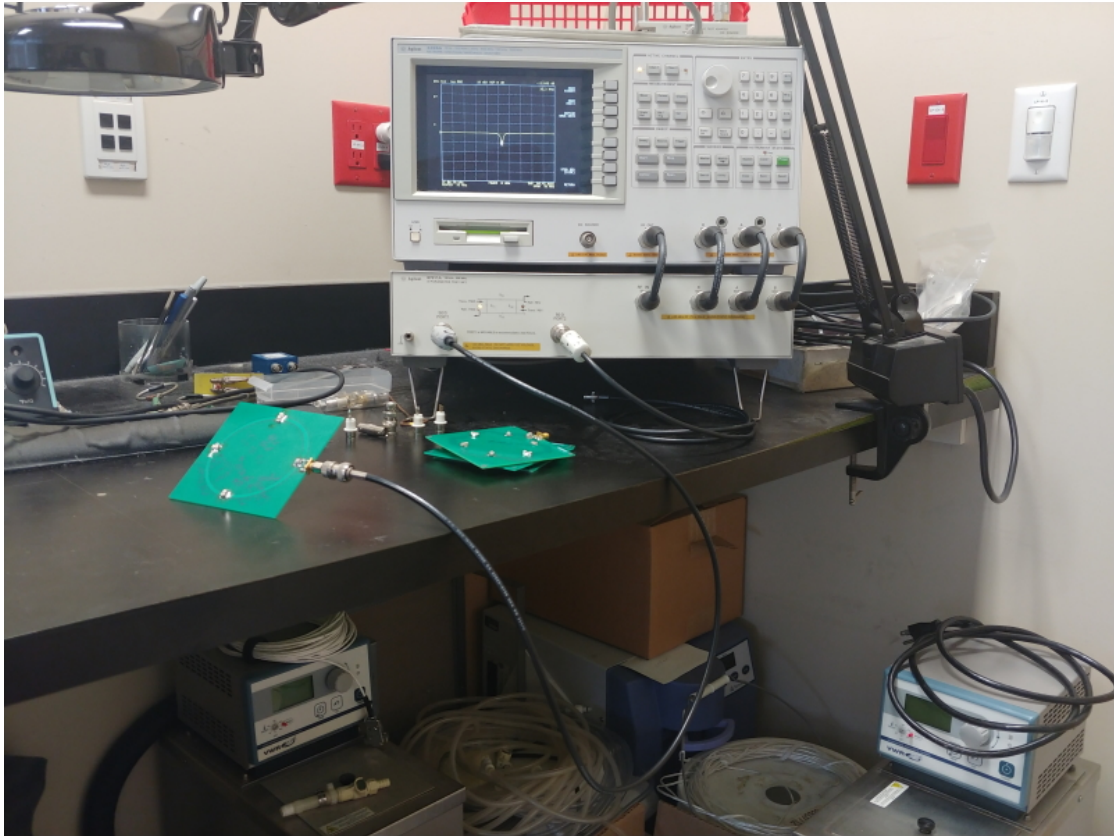
FIGURE 4.2: Image of impedance measurement setup using the Agilent 4395A
