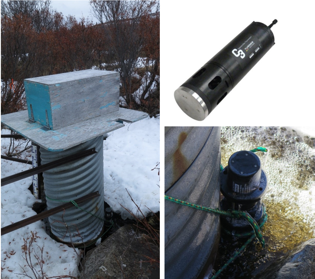
Figure 3-2. Photo of CDOM sensor deployed near Granger Creek stilling well.
