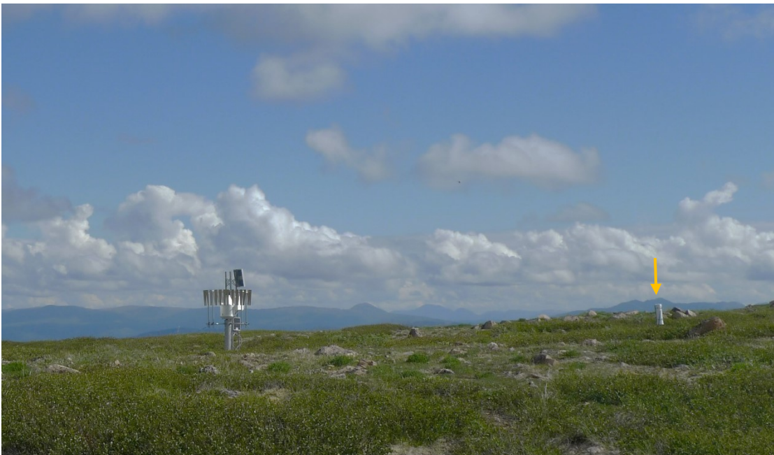
Figure 4-2. Photo of Alpine Alter-shielded Geonor total precipitation gauge and solar panel with adjacent IAEA-standard precipitation collector (shown by yellow arrow).
