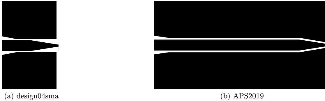
Figure 3.5: Comparison of the feed structures of the initial and final antennas. The scale is 2:1. The left side of each view is the antenna feedpoint while the right side is where the cactus-shaped radiator is connected. In the APS2019 design, the ground plane has been modified to follow the CPW taper as it meets the cactus such that the gap width remains fixed. The gap between the conductors has also been widened. These changes partly improved the broadband impedance matching.
