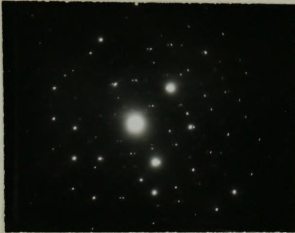
Fig. 18(c) One of the more complex electron diffraction patterns obtained from the martensitic phase.
