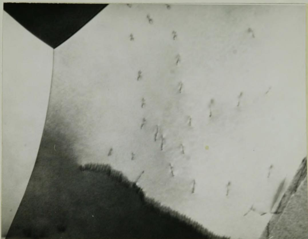
Fig. 10(a) Single phase material (51% Ni) annealed at 700°C for 15 minutes (sample H-700-1) X 25000
