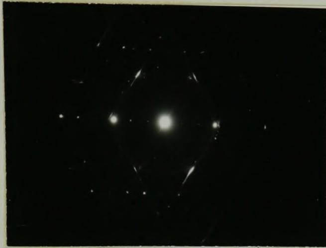
Fig. 11(b) Electron diffraction pattern showing diffraction streaks due to the coherent precipitation of a second phase (taken from H-500-2).
