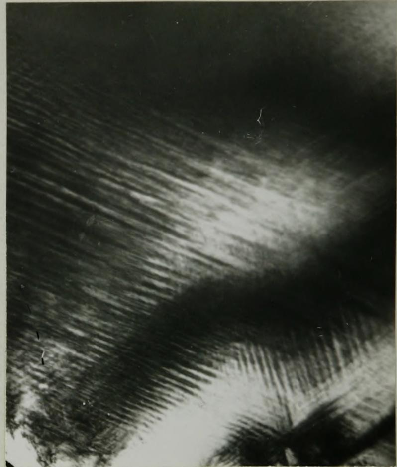
Fig. 10(b) Stripe contrast found in 51% Ni alloy annealed at 700°C for 50 minutes to 5385 minutes.
