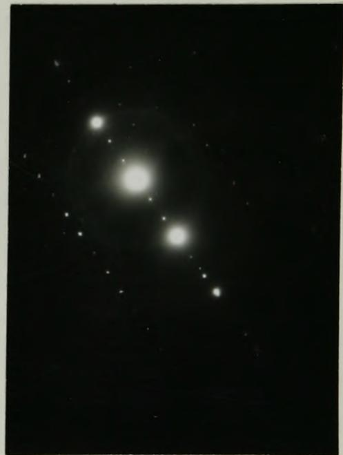
Fig. 11(c) Electron diffraction patterns showing weak super lattice spots (in addition to strong b.c.c.  $a_0 = 3.01 \text{ \AA}$  spots) which can be indexed on the basis of a  $9.03 \text{ \AA}$  simple cube (taken from H-500-3).
