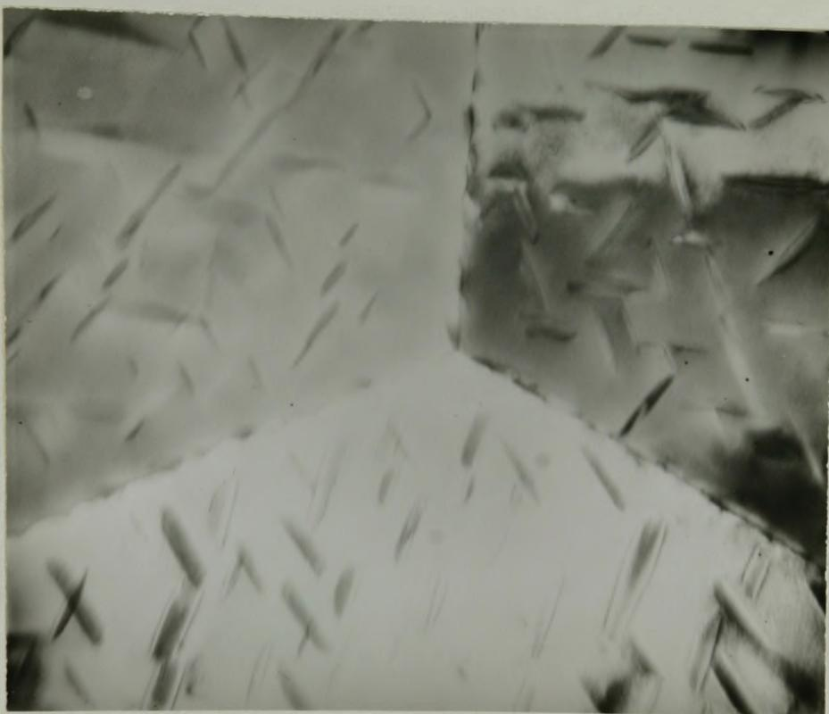
Fig. 11(a) 51% Ni alloy annealed at 700°C for 5385 minutes followed by 460 minutes at 500°C (sample H-500-2) showing coherent precipitates which are presumed to be  $Ti_2Ni$  X 30000
