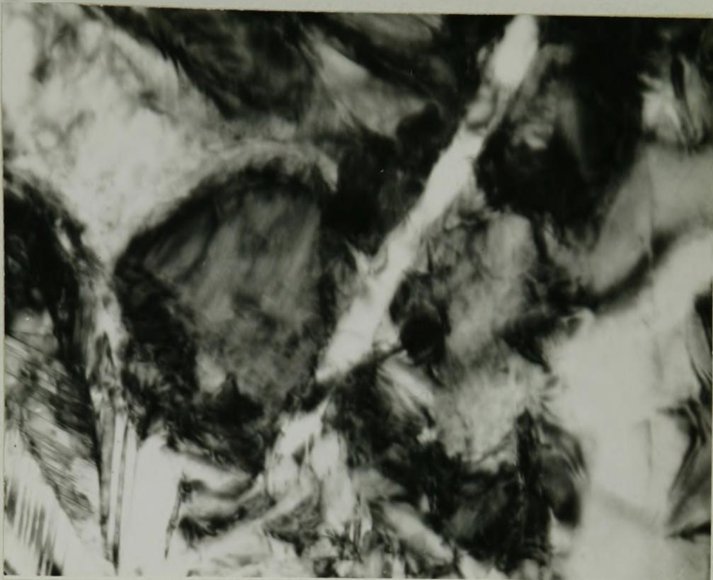
Fig. 17(a) Electron micrograph showing a  $Ti_2Ni$  precipitate and some twinned martensitic phase in a matrix of transition phase. X 94000
