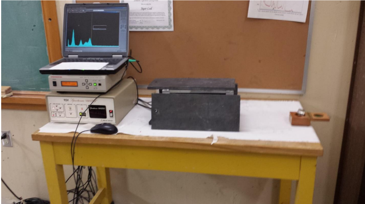
Figure 2.4: LaBr 3 (Ce) detector setup
