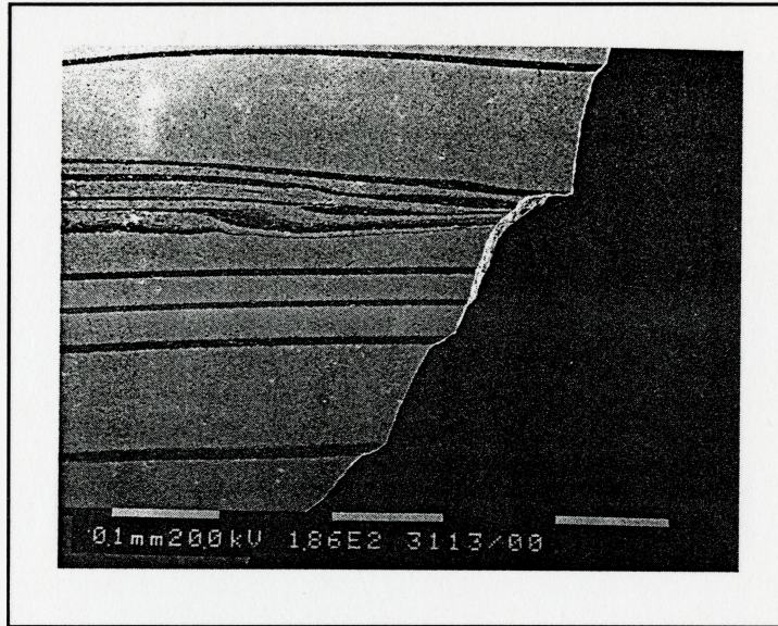
Figure 2.35 Cross-section of a fractured sample (5vol%Al 2 O 3 ) indicating deflection steps (Prakash et al , 1995).
