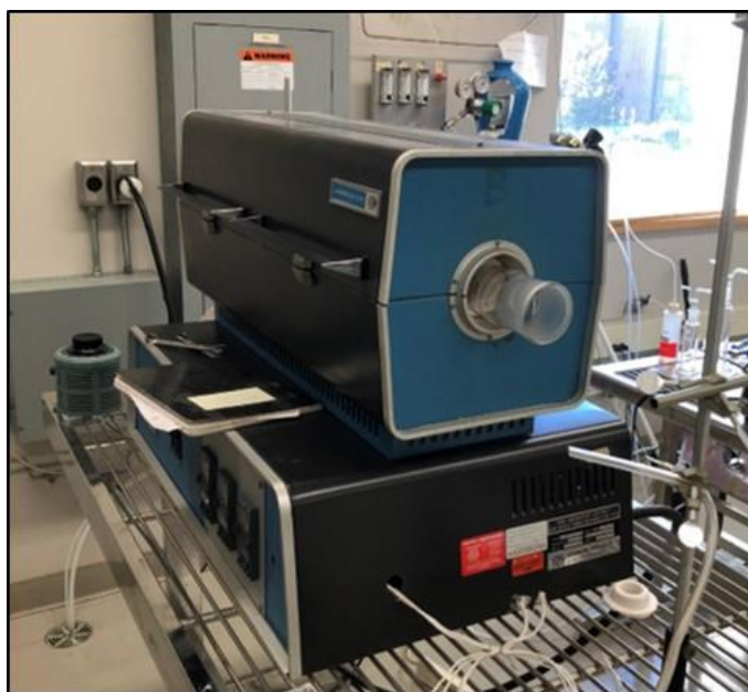
Figure 18. Quartz tube furnace for post-deposition annealing.
