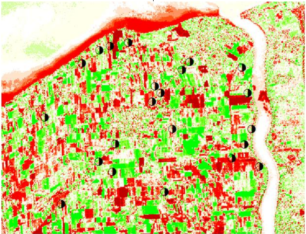
FIGURE 7: A Normalized Difference Vegetation Index (NDVI) analysis was run for the Niagara Wine growing region for August 2013 and August 2014. Changes between 2013 and 2014 are shown with increased vegetation in green, decreased in red, and negligible effects in white. The locations of the major wineries in the Niagara-on-the-Lake Region are shown.
