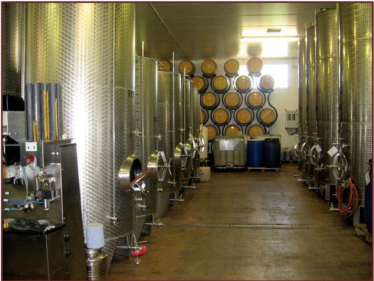
FIGURE 1: AGING VESSELS. Stainless steel tanks and oak barrels for aging wine (Wikimedia Commons, 2009).
