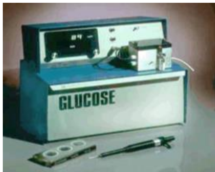
Figure. 7 The original YSI serum-glucose biosensor for diabetes clinics 1975(Turner, 2014)
