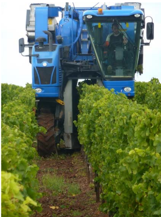
FIGURE 3: HARVESTING GRAPES. This self-propelled harvester moves over and around the grapevines, shaking them when underneath to collect the grapes as they fall. The spacing between vine rows has to be large enough to accommodate the harvesters.
