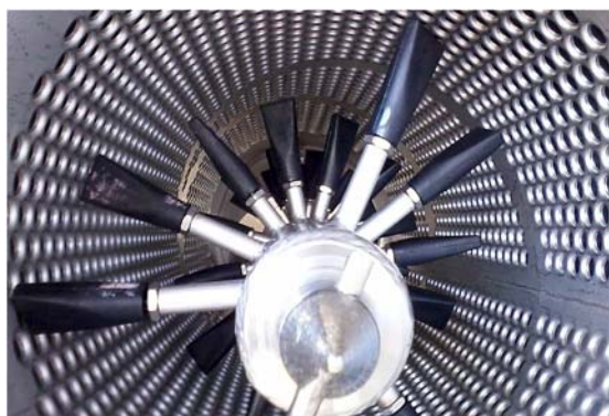
FIGURE 4: INSIDE A DESTEMMER. The destemmer consists of two components a rotating drum and the beater shaft (Colas, 2015).
