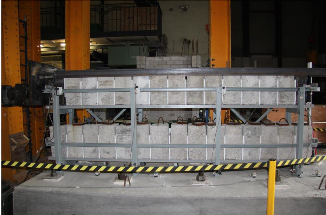
Figure 4.1: Quasi-static testing of 2-tier-1-step ABPS configuration.
