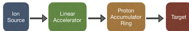
Figure 3.3: The different steps involved in neutron production at a pulsed source are shown.
