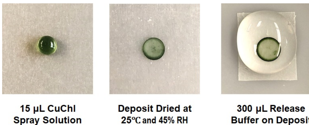
Figure 2 Photographs of the three steps in a release experiment. The spray solution composition was 0.05% CuChl + 0.01% CMC + 0.01% PAE in 5 mM phosphate buffer at pH 7.
