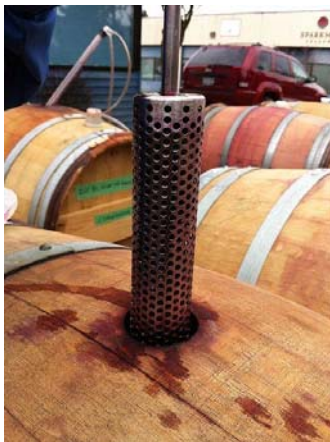
FIGURE 3: OAK INFUSER: An oak chip infuser being used in an old barrel.
