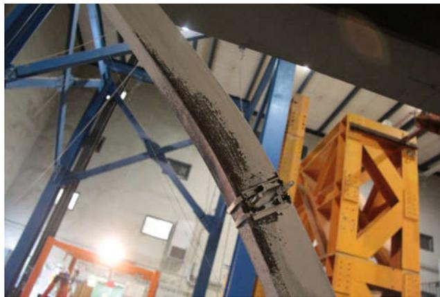
**Figure C-3** Parallel brace displacement string pots and pivot plate setup
