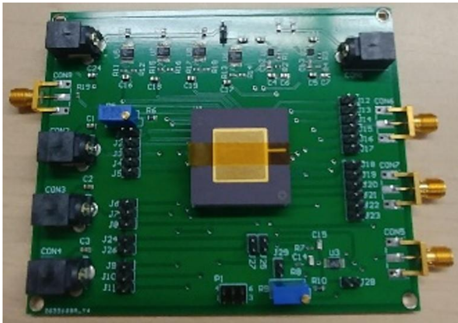
Figure 4-1: Printed circuit board (PCB) designed for testing the SPAD chips.
