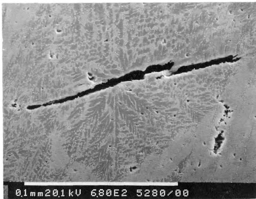
Figure 4-21b Shear bands and void growth in the Al-Ni Ohno cast alloy.
