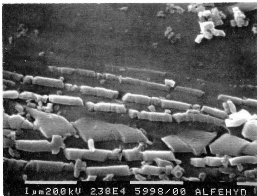
Figure 4-15 SEM micrograph of the Al-Fe OCC after hydrostatic extrusion.
