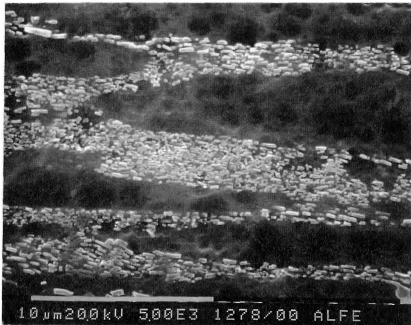
Figure 4-11 Swaged Ohno cast Al-Fe alloy.
