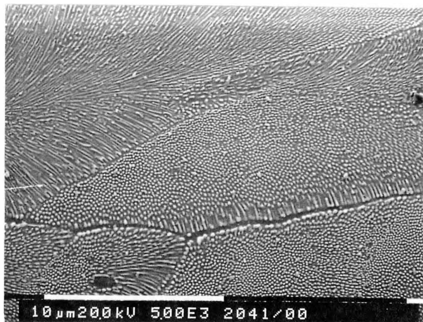
Figure 4-4 Regions of Al-Al 3 Ni eutectic deviating from the growth direction.
