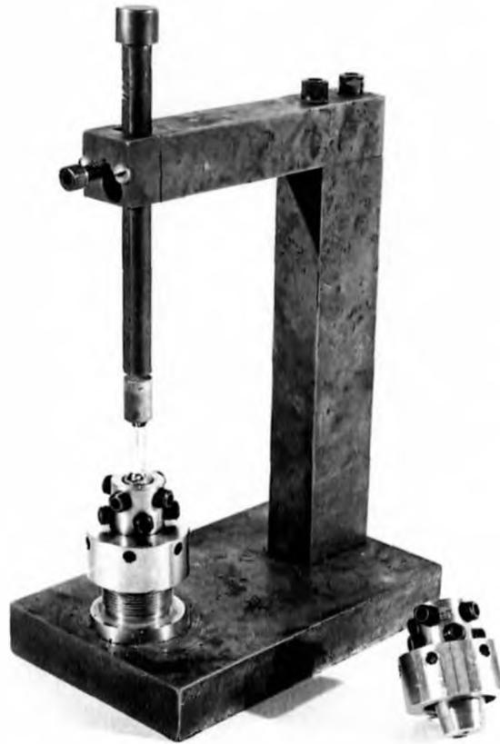
Figure 3.8 Alignment rig used to set-up the specimens in the grips.
