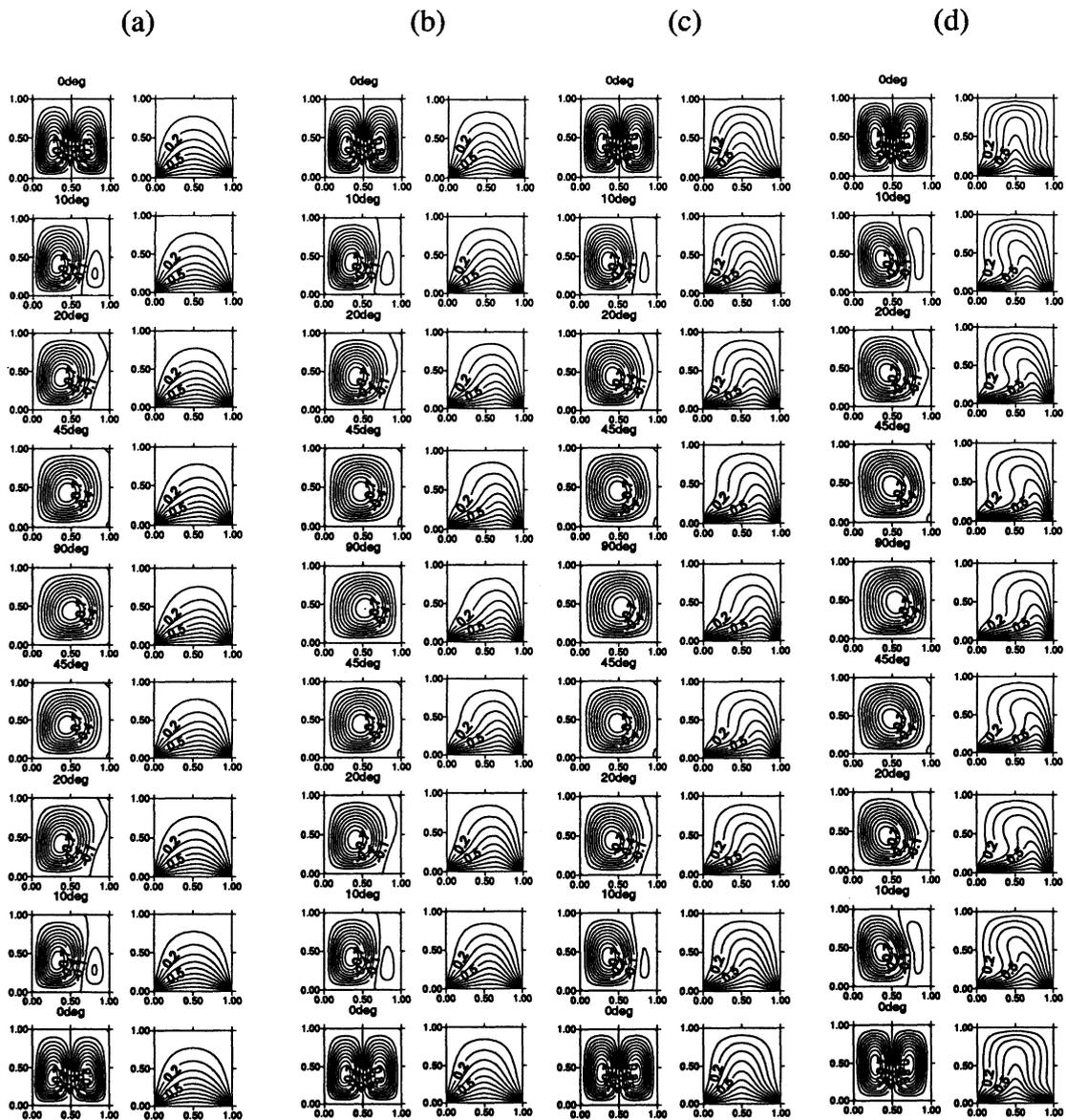
Fig. 3.17 Normalized streamlines and isothermal lines for CC configuration at various angles of inclination and four Ra numbers. (a) Ra=1000, (b) Ra=3000, (c) Ra=5000, (d) Ra=10<sup>4</sup>. Positive values indicate rotation in clockwise direction.
