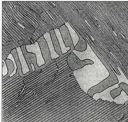
Fig.1.8 Transverse section of unidirectionally grown polycrystalline eutectoid Co-Si showing discontinuous coarsening after annealing at 1273K for 96 hours. The lower grain has invaded the upper grain on the left and the upper grain has invaded the lower grain on the right- in both cases the invaded grain has its lamellae most nearly normal to the grain boundary. Note the large ratio ( r' ) of lamellar spacing after growth to that before. (After Livingston and Cahn, 1974).
