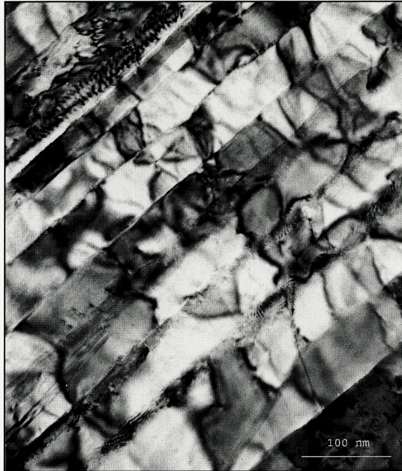
Fig.3.6 Cross-sectional TEM bright field images for Au/Pt multilayers prepared by the repeated rolling/folding after 110passes. Regular multilayers are observed locally.
