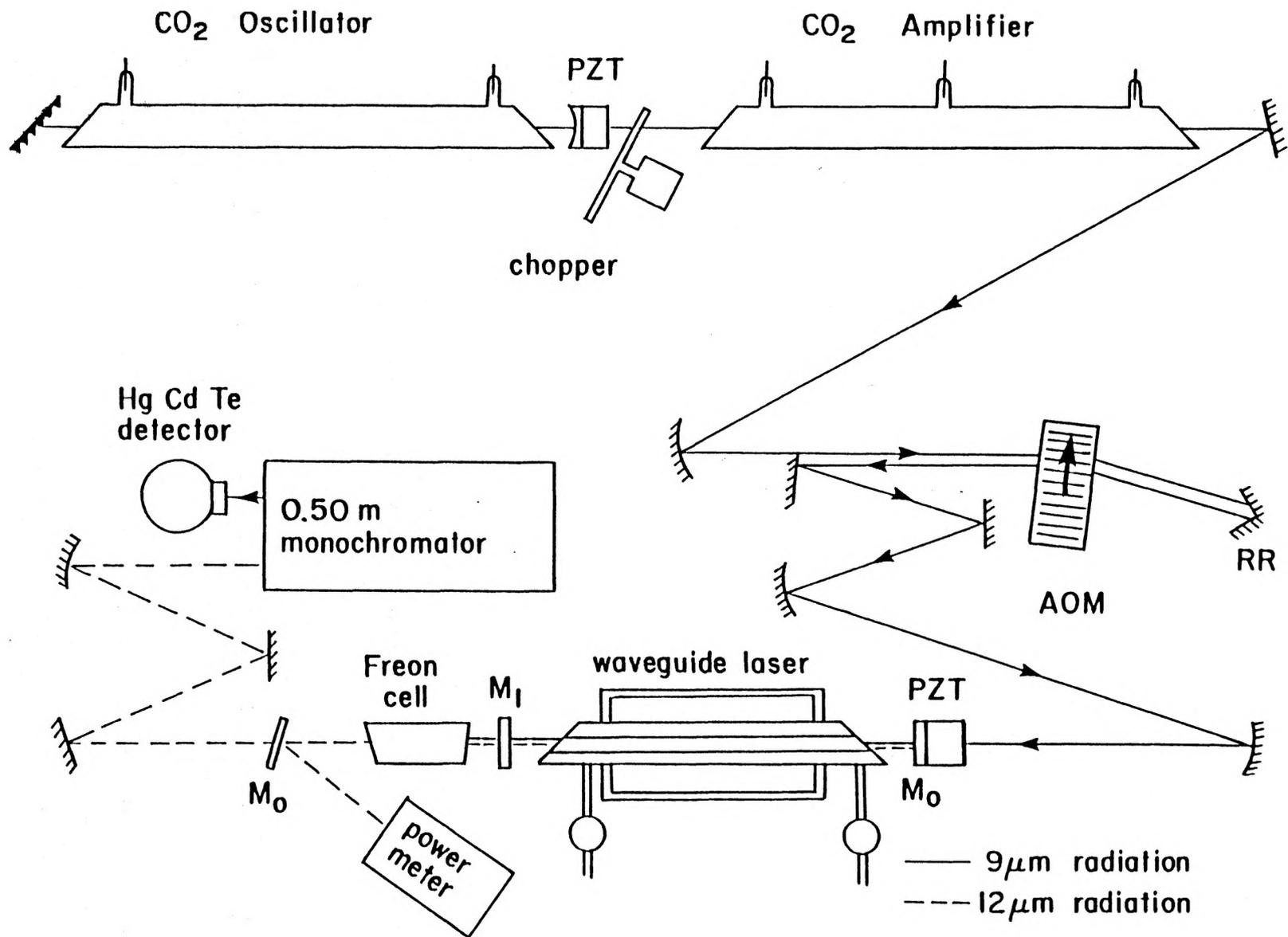
the 12- $\mu\text{m}$  output was taken from a mirror at the other end of the cavity. The output beam passed through a Freon-12 cell, which removed the residual 9- $\mu\text{m}$  radiation, and was then directed to the Scientec power meter. Identification of the lasing wavelength was made using a 0.5 m monochromator.
