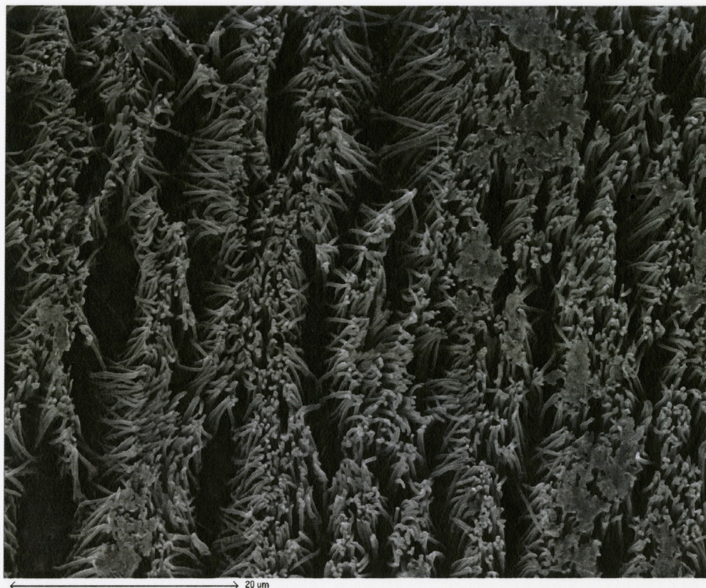
Figure 4.3 Scanning electron micrograph of free nanocylinders which were template-synthesized within the pores of a 200 nm polycarbonate membrane.
