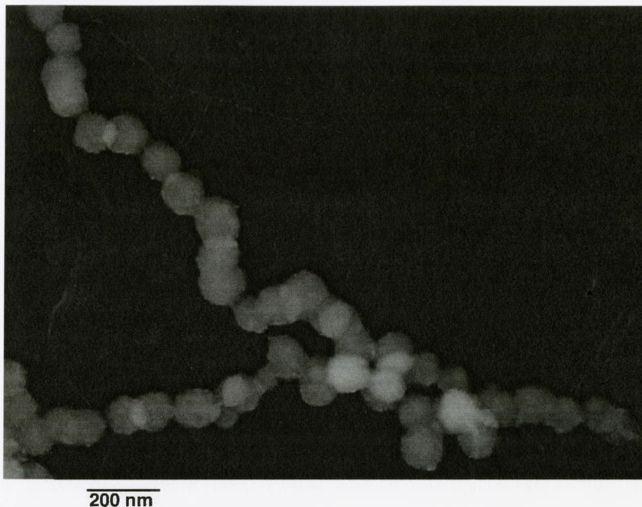
Figure 4.17 Transmission electron micrograph of two freed nanostructures which were template-synthesized in a 20 nm alumina membrane.
