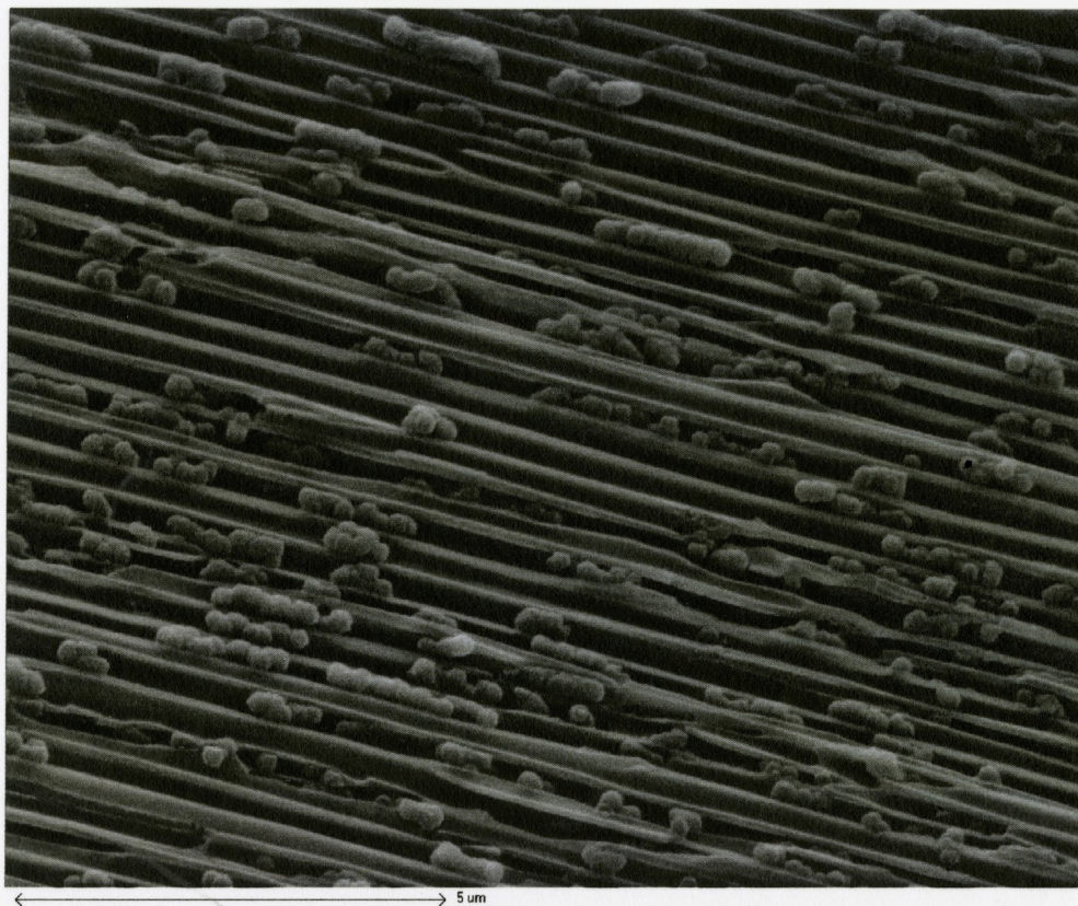
Figure 4.14 Edge-on scanning electron micrograph of a polypyrrole-filled 100 nm alumina membrane.
