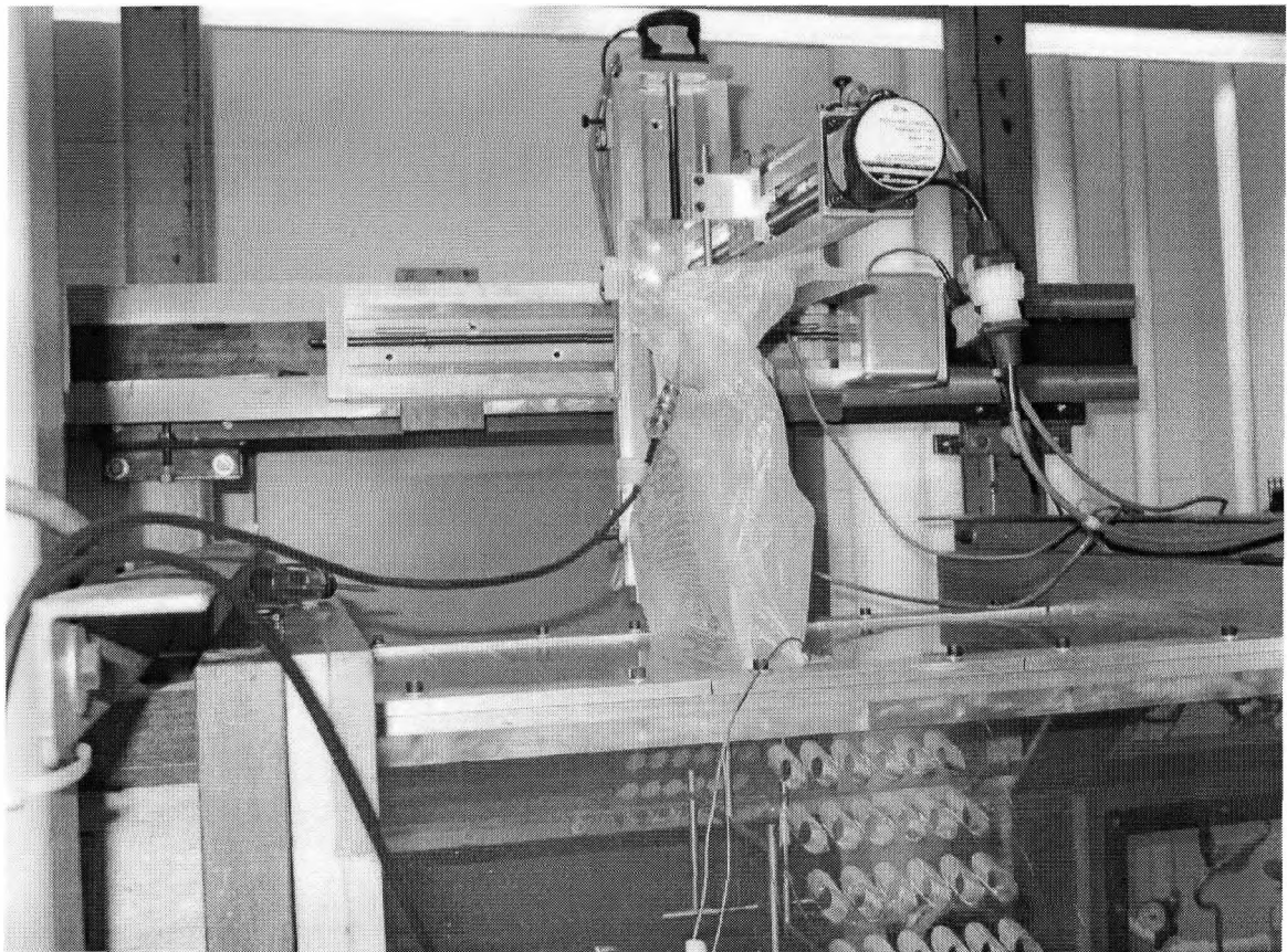
Figure 3.8: Traversing mechanism position above the test section.
