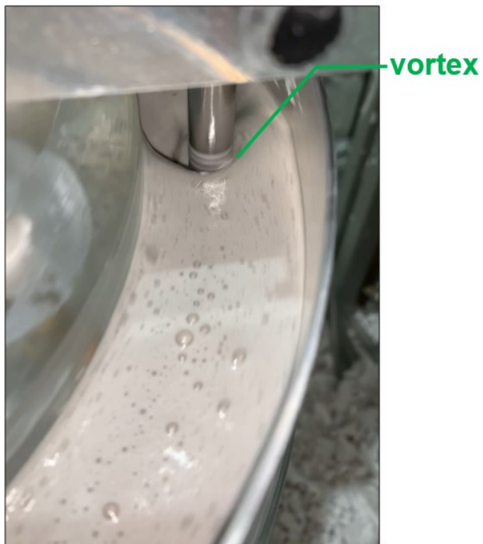
Figure 4.28: Vortex Formation at High Spindle Speed.
