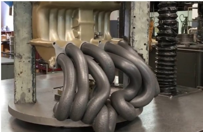
Figure 1.6: (a) Extrusion Honing of an Engine Manifold with a Non-Newtonian Abrasive Putty [14] (b) Body Armor Absorbing the Momentum of a Bullet [15].
