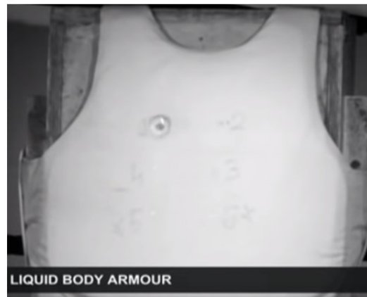
Figure 1.6: (a) Extrusion Honing of an Engine Manifold with a Non-Newtonian Abrasive Putty [14] (b) Body Armor Absorbing the Momentum of a Bullet [15].
