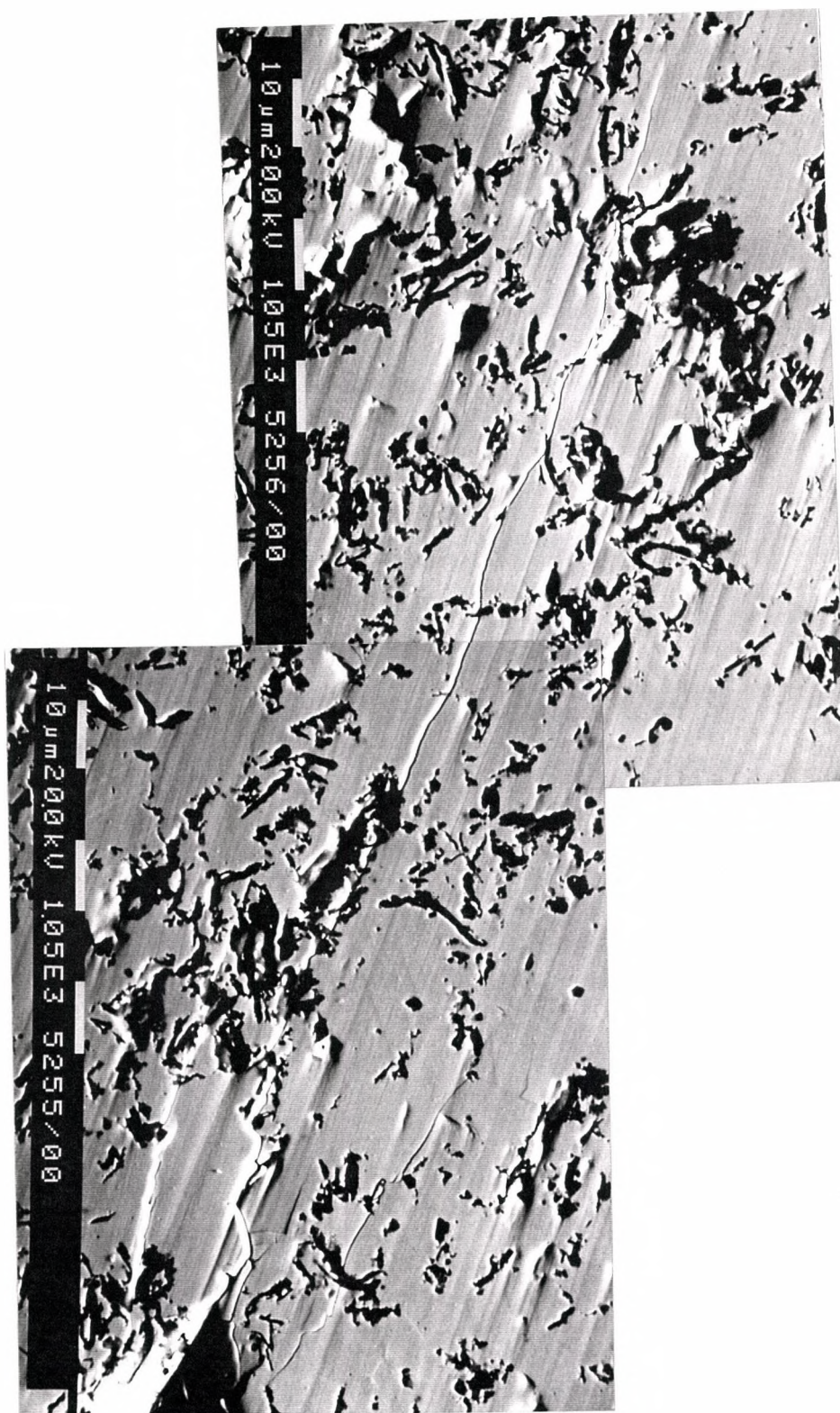
Figure 4-20: Crack propagation in 20 vol% SiC-MoSi 2 .
