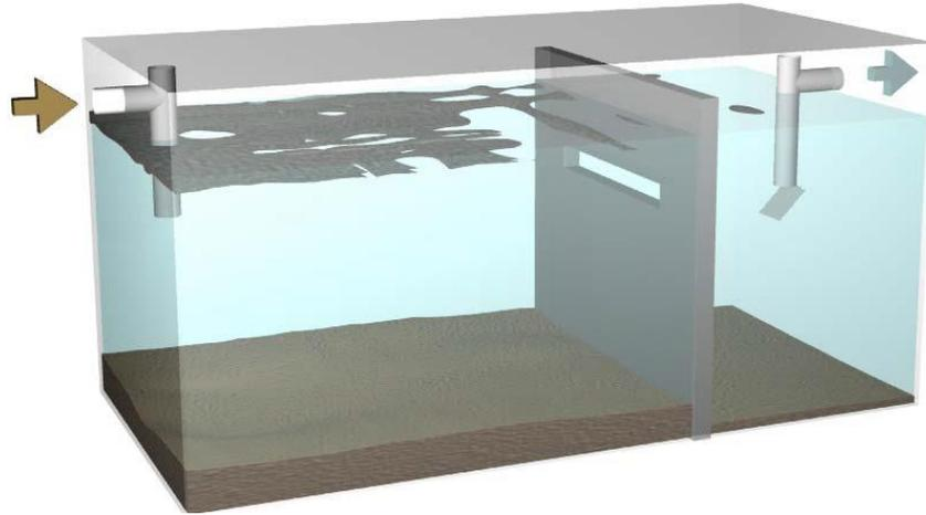
**Figure 1: Flow through a conventional septic tank (WBS, 2009).** The yellow arrow indicates the influent entry point and the light blue arrow indicates the effluent exit point. Scum and settled solids are shown at the top and bottom of the septic tank, respectively (Section 1.2).
