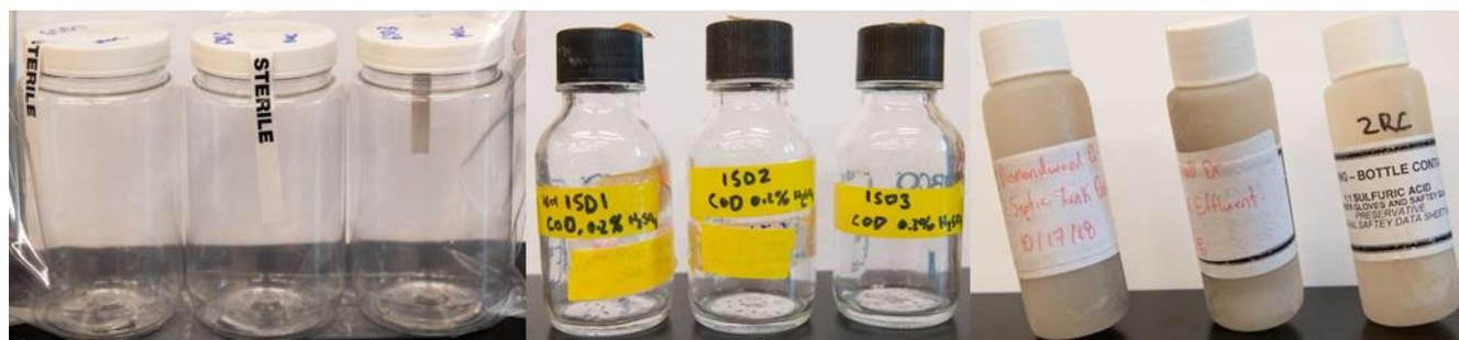
**Figure 1: 500 ml (left), 100 ml glass (middle), and 100 ml plastic (right) sampling bottles. 100 ml glass and plastic sampling bottles are preloaded with sulfuric acid preservative.**
