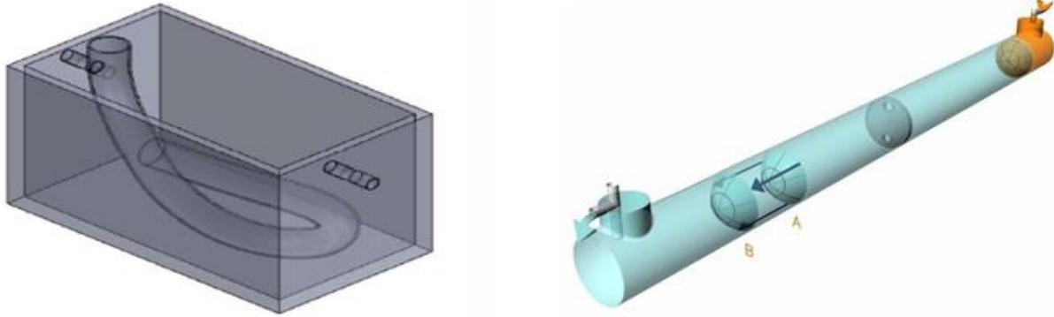
**Figure 4: An InnerTube septic tank system (left) and a plug flow reactor (right).** The arrows in the plug flow reactor diagram indicate the direction of flow and ‘plug’ movement (Jowett, 2017) (Section 2.1.2, 2.1.3).
