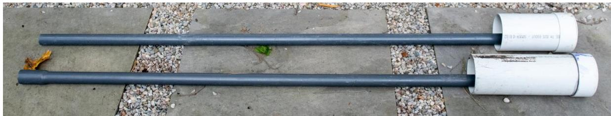
**Figure 2: Effluent sampler (top) and collection vessel (bottom).**
