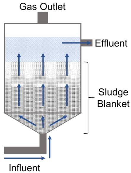
**Figure 5: Upflow anaerobic sludge blanket (UASB) reactor.** The sludge blanket is comprised of granules containing microbial communities capable of anaerobic digestion. Arrows indicate the direction of wastewater flow (Section 2.1.5).
